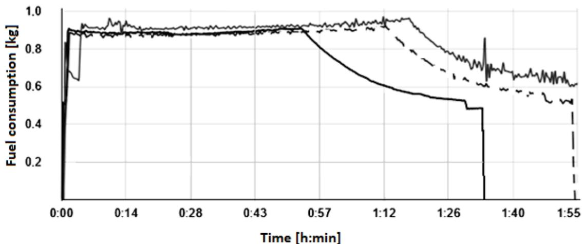
Fig. 2. Power generator momentary fuel consumption (kg/h) for three different fuels: Diesel (black) F-34 (black dashed) and Jet A-1 (grey)
