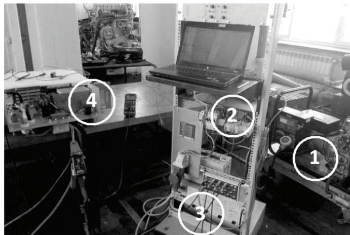
Fig. 1. Charging test stand: 1 – power generator, 2 – current-voltage parameters acquisition system
