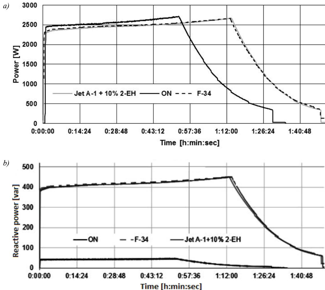
Fig. 3. Battery charging process: a) active power of generator powered with Diesel (black line) F-34 (black dashed) and Jet A-1 (grey); b) reactive power of generator powered with Diesel (black line), F-34 (black dashed) and Jet A-1 (grey)
