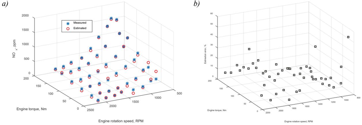
Fig. 8. Operation of the trained neural network, a) comparison of estimated and measured values, b) estimation error
