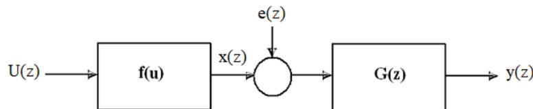
Fig. 3. Hammerstein model flowchart
