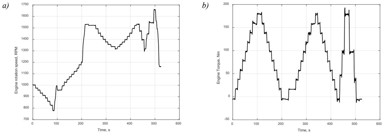
Fig. 10. Measurement results for registered evaluation trials: a) engine rotation speed, b) engine torque
