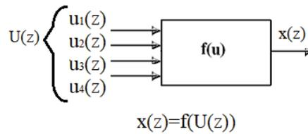
Fig. 4. Non-linear element of the Hammerstein model
