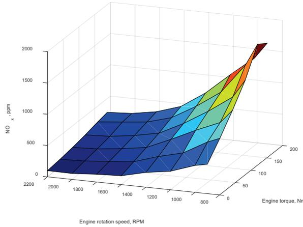
Fig. 6. NOx emission map for static points
