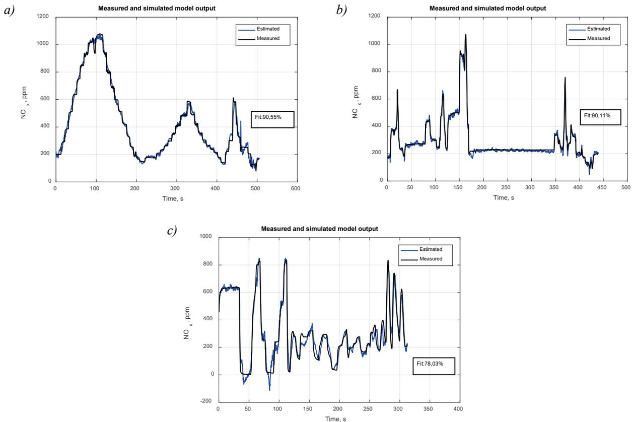
Fig. 11. Comparison of experimental and modelled data for nitrogen oxide emissions
