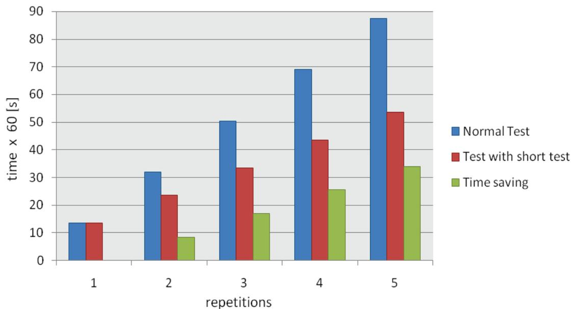
*Fig. 3. Summary of the time of full regeneration of the injector A and number of repetition cycles using test with a short diagnostic test*
