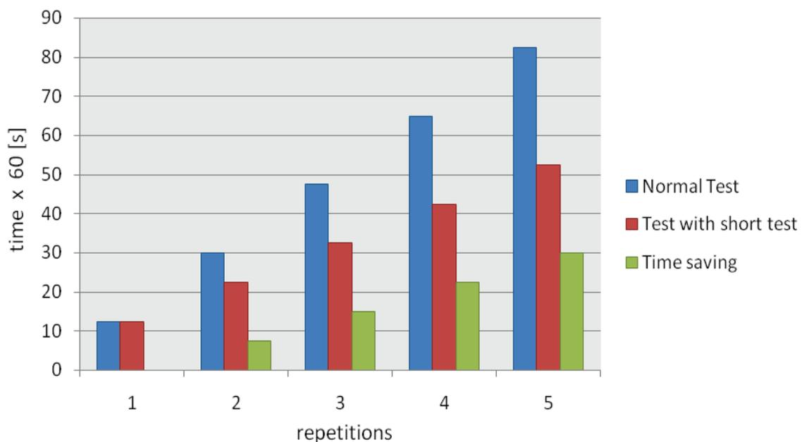
*Fig. 4. Summary of the time of full regeneration of the injector B and number of repetition cycles using a short diagnostic test*
