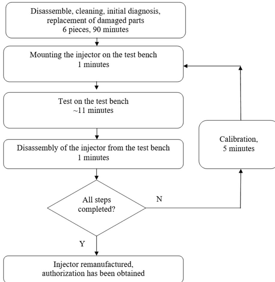
*Fig. 2. Diagram showing the steps necessary to carry out the regeneration of the injector and the times of performing individual operations*
