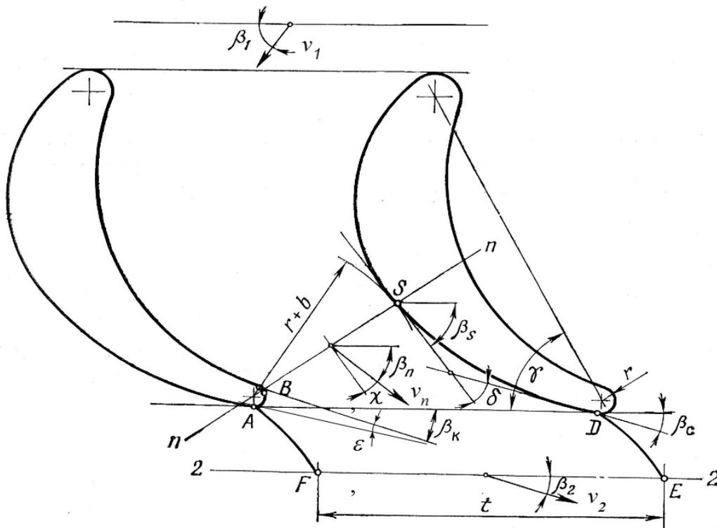
Fig. 1. Design angles of a blade row in its exit region, defined for a turbine design point [4]
