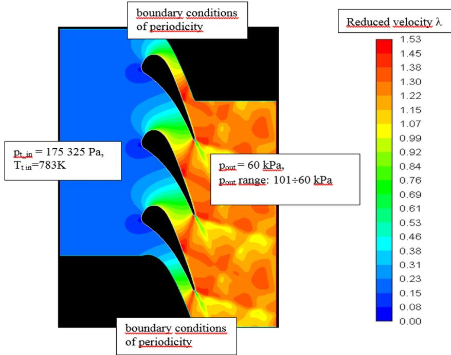
Fig. 2. Boundary conditions applied in CFD analysis and contour of reduced velocity  $\lambda$  in flow solution with supercritical exit conditions
