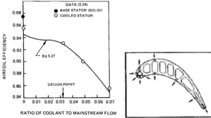
Fig. 4. Decrease of airfoil efficiency due to streams emanating from blade surface according to [8]. The solid line shows results of eq. (7)
