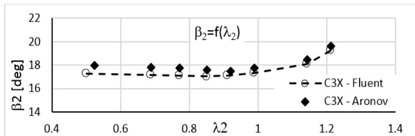
Fig. 3. Comparison of gas exit angle  $\beta_2$  obtained in the numerical solution of viscous flow with results of analytical formulas for different values of reduced velocity  $\lambda_2$
