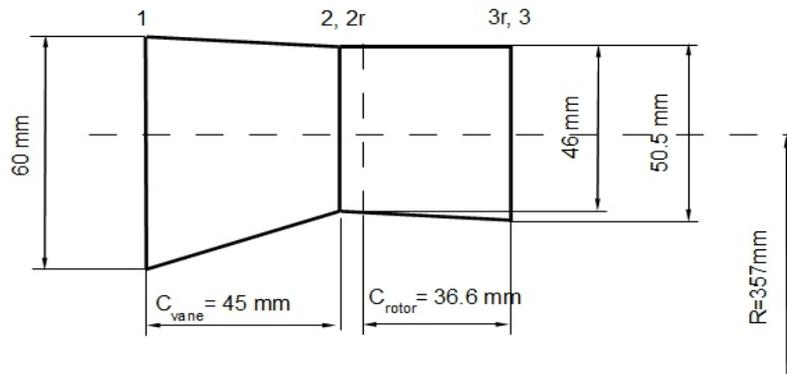
Fig. 6. Flow-path dimensions of the test turbine stage
