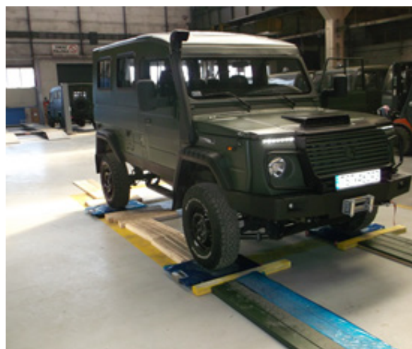
Fig. 6. Honker M-AX car on measuring platform
