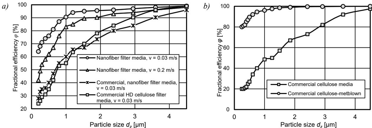
Fig. 3. a) Pleated filter elements made of cellulose fibres, nanofiber layer, and cellulose fibres filtration efficiency [14], b) air filtration effectiveness for various dust grains sizes at a flow rate of  $0.03\ \text{m/s}$  [10]
