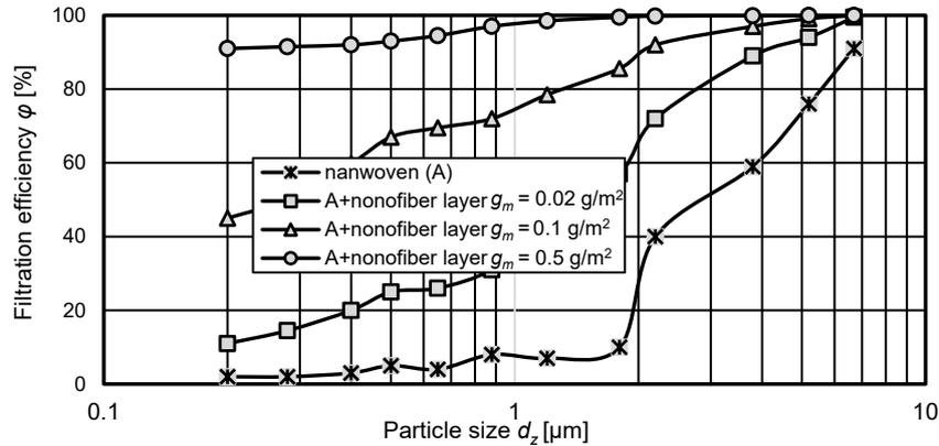
Fig. 6. Material filtration effectiveness (nonwoven fabric sample A) without a nanofiber layer, and with nanofiber layer with unit weight  $g_m = 0.02 \text{ g/m}^2$ ,  $g_m = 0.1 \text{ g/m}^2$ ,  $g_m = 0.5 \text{ g/m}^2$  [12]
