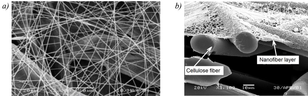
Fig. 2. Nanofibers applied to a cellulose substrate: a) top view, b) cross-section view [11]
