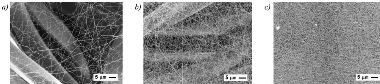
Fig. 5. SEM microscope photographs for sample C with nanofiber a basis weight layer: a)  $g_m = 0.02 \text{ g/m}^2$ , b)  $g_m = 0.1 \text{ g/m}^2$ , c)  $g_m = 0.5 \text{ g/m}^2$  [12]
