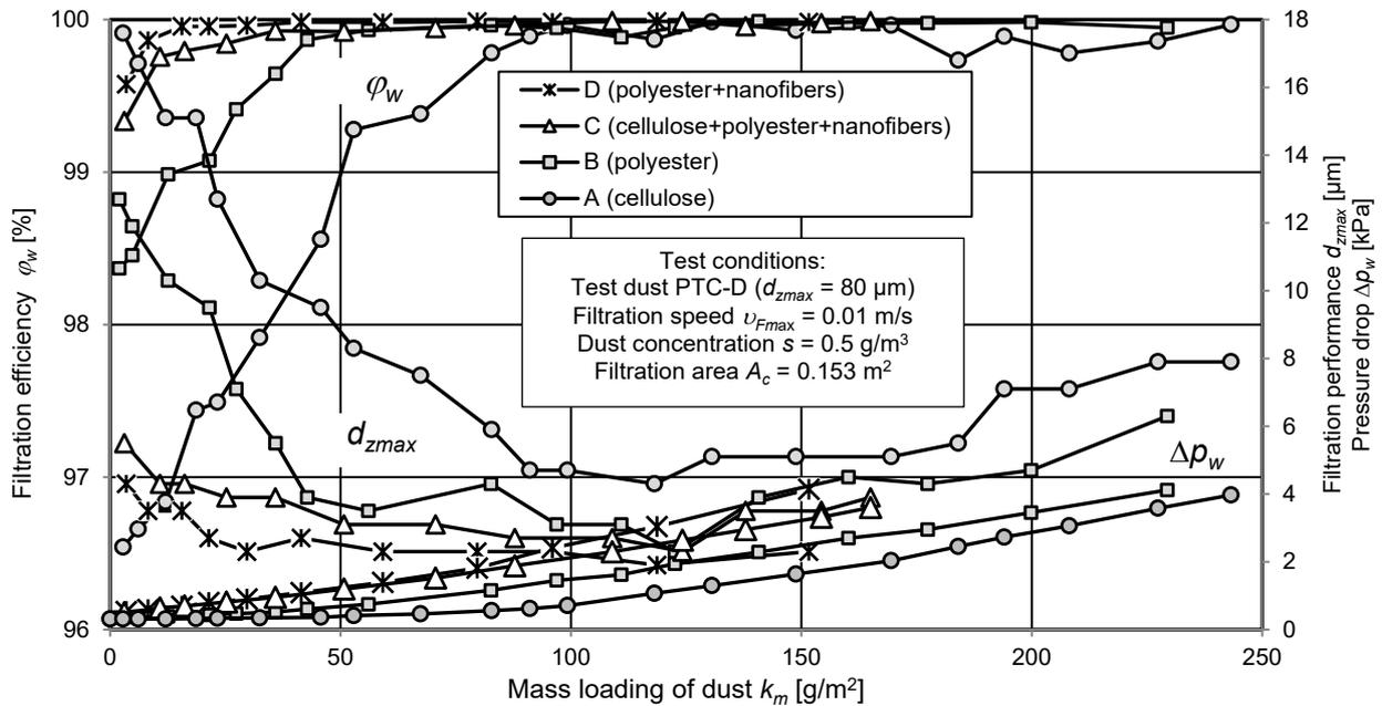
Fig. 9. Filtration efficiency  $\varphi_w$ , filtration performance,  $d_{zmax}$ , and pressure drop  $\Delta p_w$  depending on the tested filter cartridges dust mass loading  $k_m$
