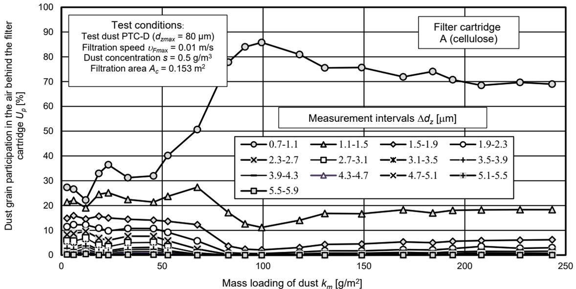
Fig. 11. Dust grains granulometric composition, which passed through filter cartridge A (cellulose)
