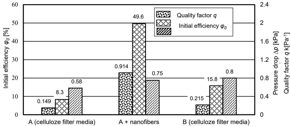
Fig. 4. Standard filtration materials effectiveness used in car air filters, and standard filtration material with a thin layer of electrospinning fibres [9]
