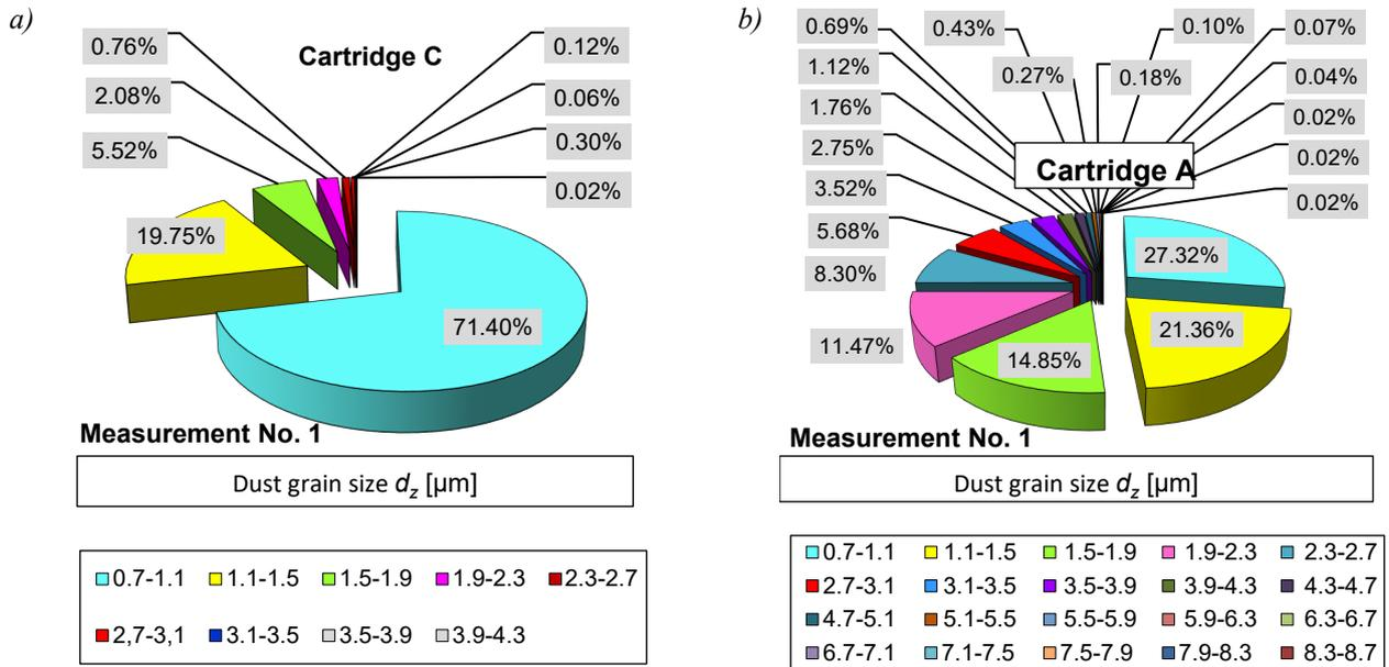
Fig. 10. Granular composition of dust grains assumed by the filter cartridge: a) cartridge C (cellulose+ polyester nanofibers) after reaching dust mass loading  $k_m = 3 \text{ g/m}^2$ , b) cartridge A (cellulose) after reaching the dust mass loading  $k_m = 2.8 \text{ g/m}^2$
