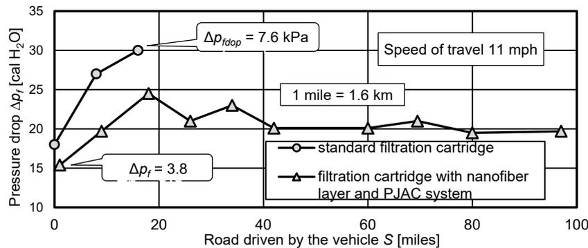
Fig. 7. Air cleaner pressure drop versus miles travelled in 20 mph convoy test in desert conditions and automatic cleaning system [10]
