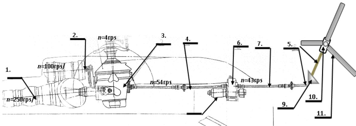
Fig. 2. The location of transmission elements between engine and generator on the multi-purpose helicopter: 1 – powerplant, 2 – mechanical fan, 3 – main gearbox, 4, 5, 7 – power transmission shaft, 6 – generator power gearbox, 8 – left generator (behind it, to the same power and accessory gearbox a right generator is mounted), 9 – intermediate tail rotor gearbox, 10 – tail rotor gearbox, 11 – tail rotor
