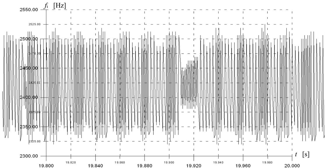
Fig. 4. Modulations of instantaneous frequency in time function during spatial resonance between the worn upper bearing of the main gearbox and worn bearing supports of Z30 toothed wheel in generator power gearbox
