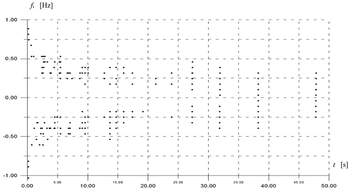
Fig. 3. Characteristic sets acquired for the powerplant of "negative standard" of the multi-purpose helicopter with damaged upper bearing of the main gearbox
