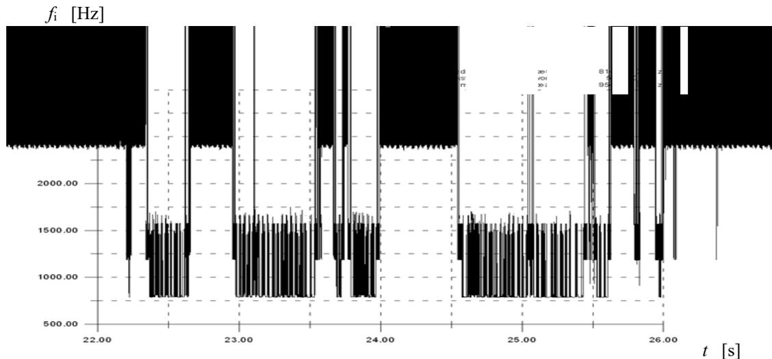
Fig. 7. The rupture of one-way clutch of the helicopter – the imaging obtained by the application of FAM-C method
