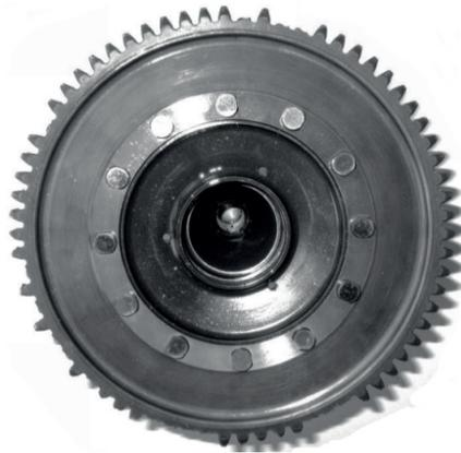
Fig. 5. Z30 toothed wheel with broken teeth
