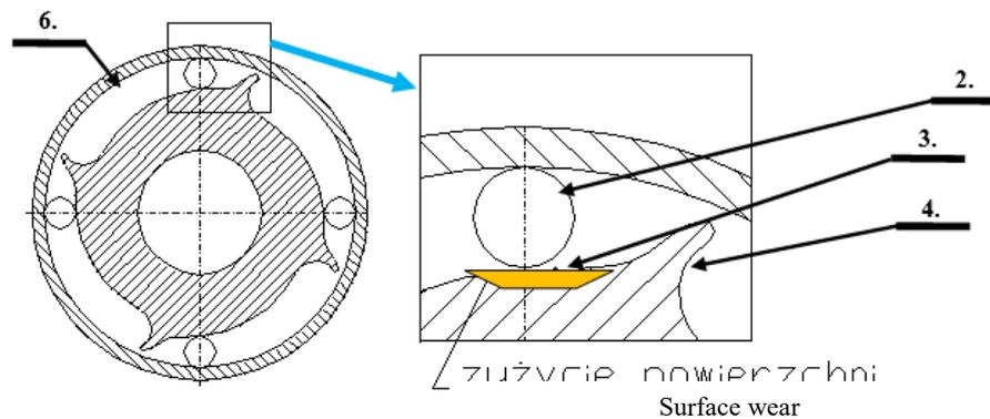
Fig. 6. One-way clutch – pictorial diagram:
