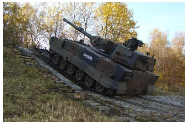
Fig. 5. The test station a) lateral inclination angle (M1A2 Abrams tank) [2], b) approach angle (ANDERS platform) [3]
