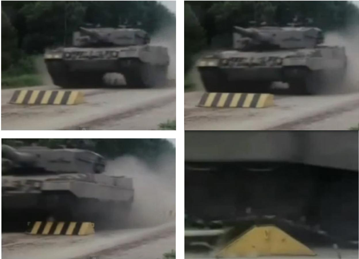
Fig.3. The Leopard 2 tank – the sequences of driving on the transverse unevenness with a trapezoidal outline with a high velocity [1], four shots that show an operation of the suspension and the caterpillar mechanism.
