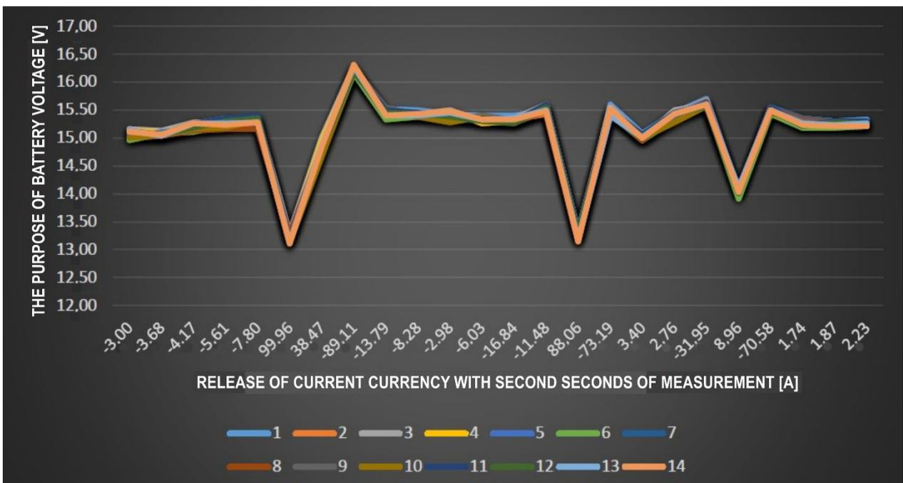
Fig. 6. Voltage values of individual HV battery cells
