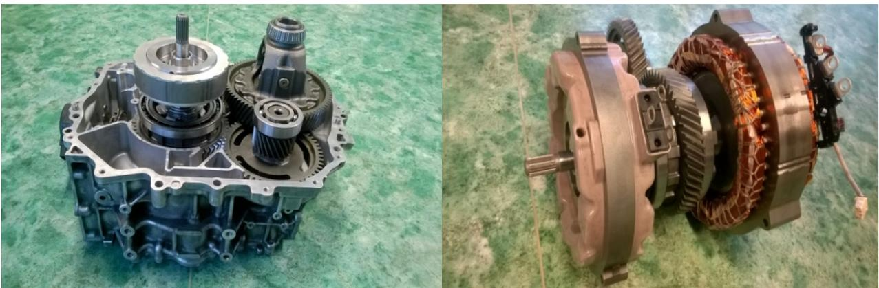
Fig. 2. Electronically controlled continuously variable transmission (eCVT)[8]
