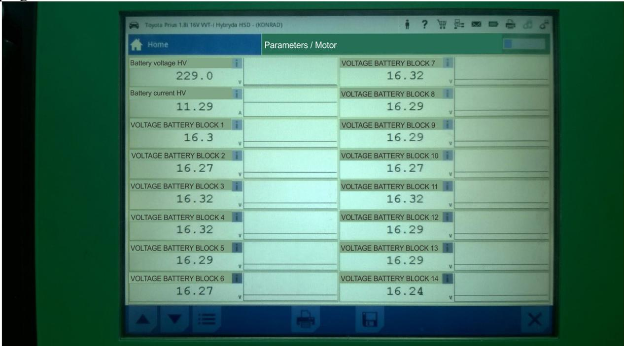
Fig. 5. Current parameters of the HV battery [8]
