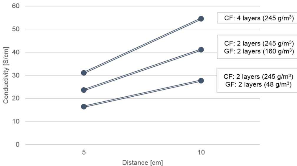
Fig. 7. Electrical conductivity depending on the distance between electrodes, CF density of 245 g/m<sup>3</sup>
