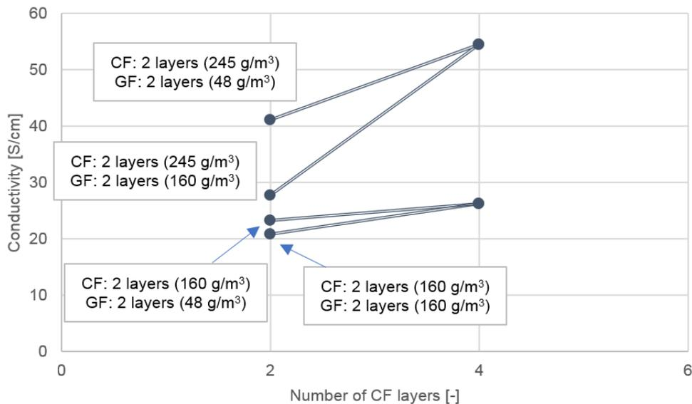
Fig. 4. Electrical conductivity as a function of number of CF layers, I orientation (0°)
