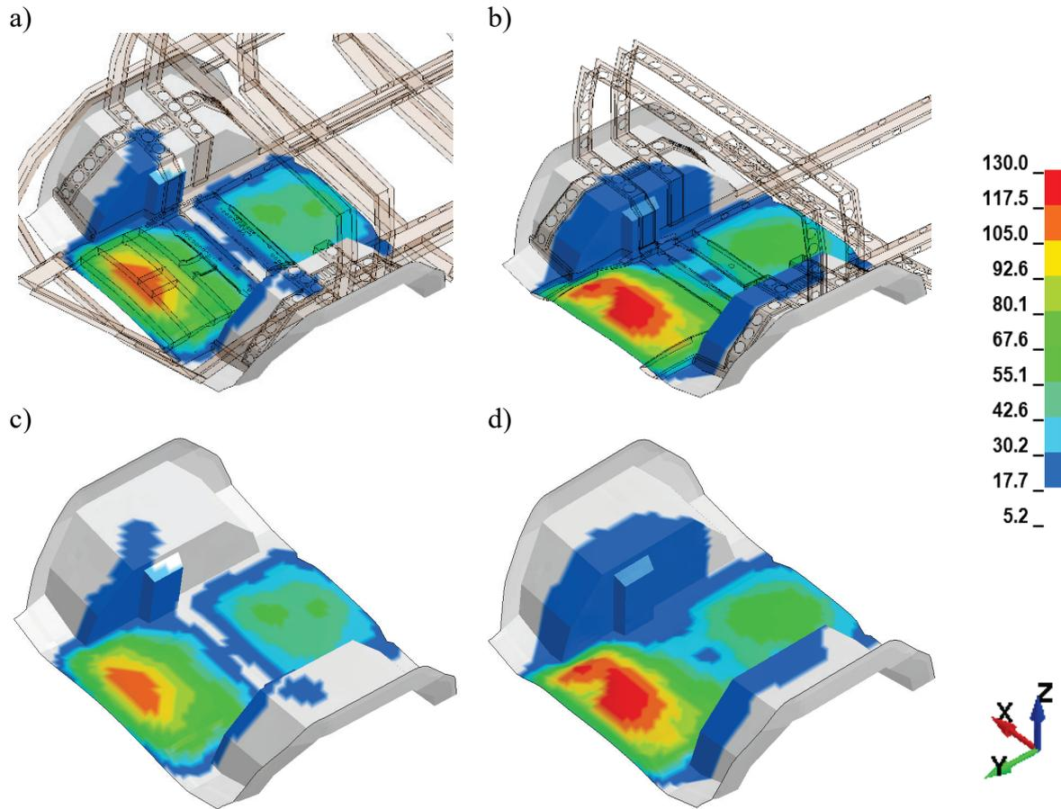
*Fig. 7. Vertical displacement on "z" [mm] of the system for a selected moment of time  $t = 4$  ms. Charge mass 20 kg of TNT a), c) system after modification b), d) reference system (before modification)*
