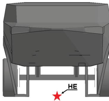
Fig. 6. Location of the explosive material in respect to the vehicle
