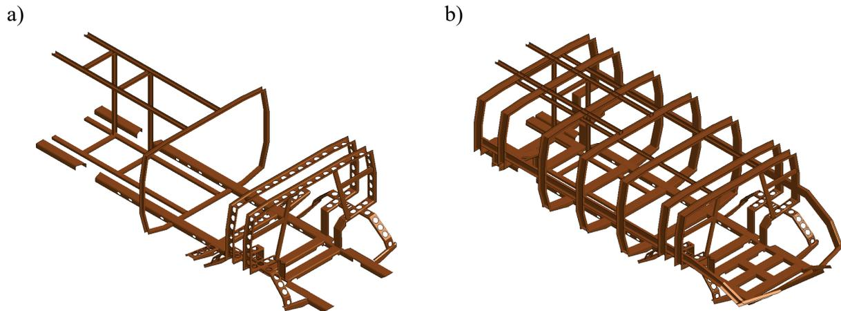
Fig. 5. System of the internal space frame improving the supporting structure stiffness a) before modification, b) after modification
