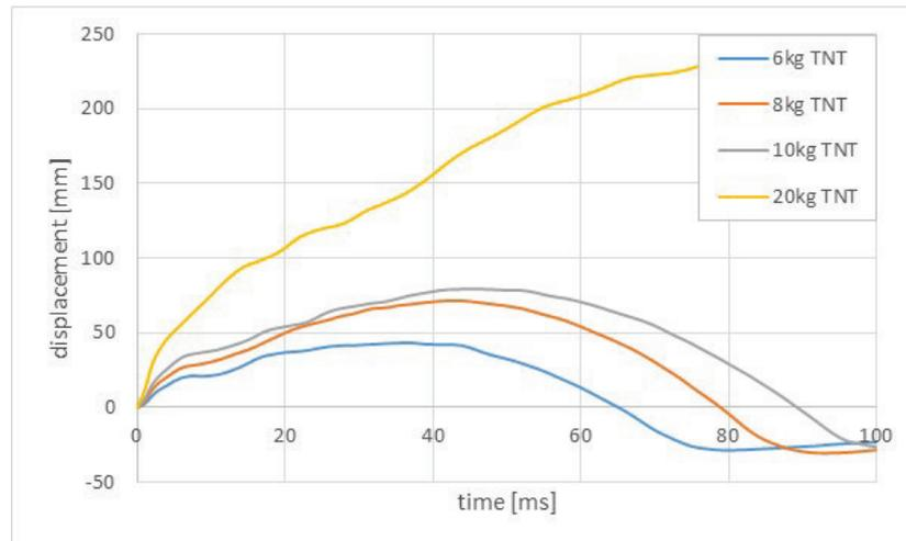
Fig. 9. Displacement of the floor plate centre of gravity for the modified system
