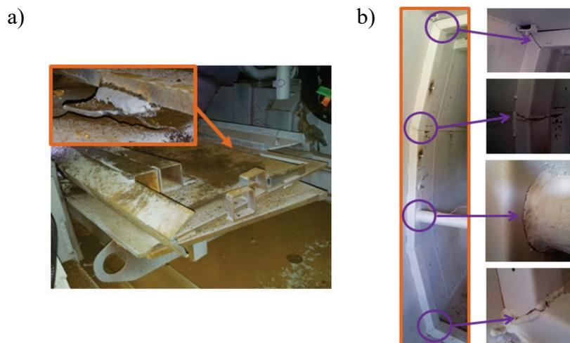
Fig. 3. Damage inside the vehicle resulting from experimental tests
