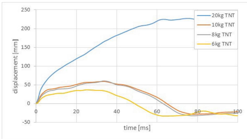
*Fig. 8. Displacement of the floor plate centre of gravity for the reference system (before modification)*
