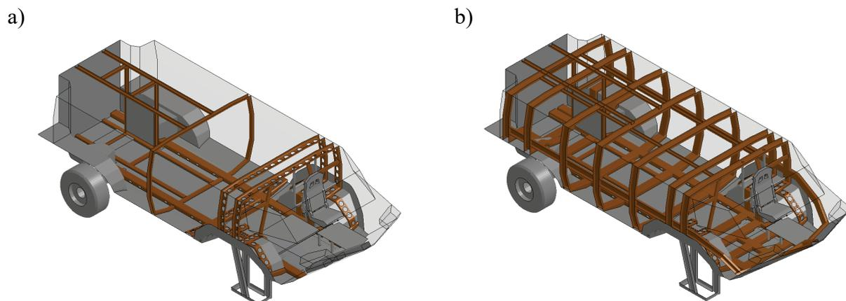
*Fig. 4. View of the supporting structure with a modified suspension system a) supporting structure before modification, b) supporting structure after modification*
