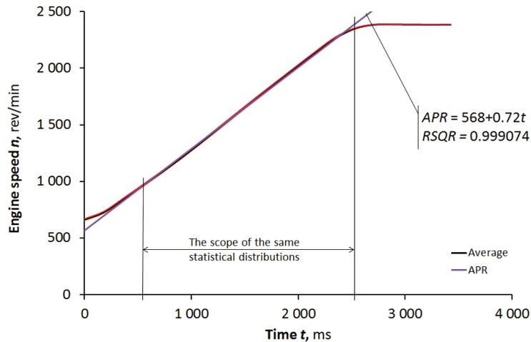
Fig. 9. Average speed curve of the run-up and a simple approximation of its values described by normal distribution
