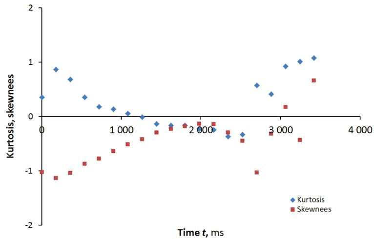
Fig. 7. Kurtosis I skewness of speed distribution in particular moments of the run-up
