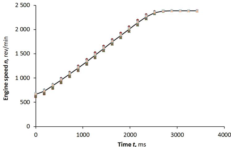
Fig. 5. The recorded values and the course of the average engine speed values in relation to the time of acceleration (run-up) of the engine
