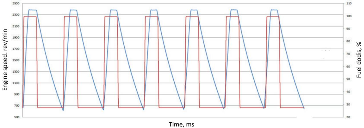
Fig. 4. The course of fuel dose and engine speed during measurements
