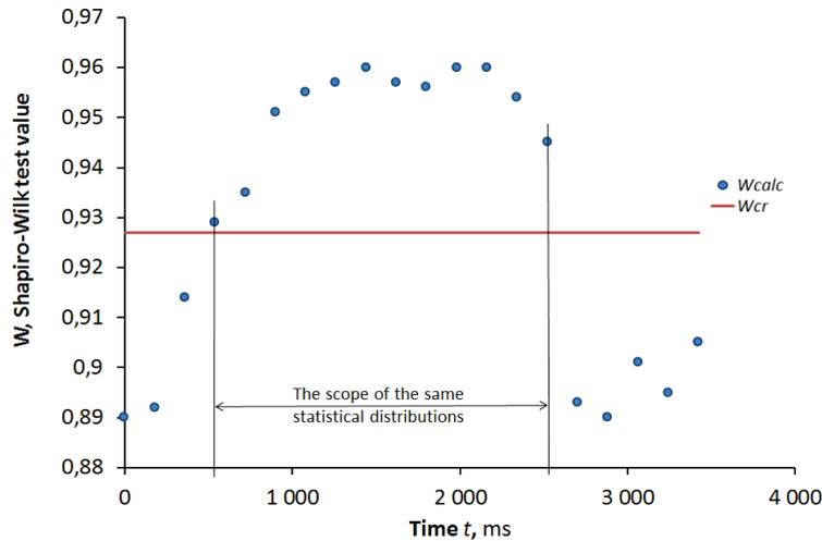
Fig. 8. Values of the Shapiro-Wilk distribution statistics in particular times of the run-up
