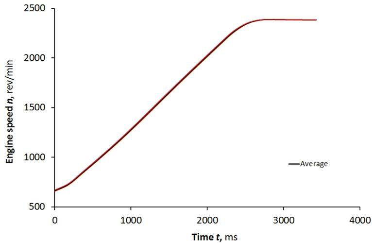
Fig. 6. The course of the mean value (with its confidence interval) of the engine speed during its run-up
