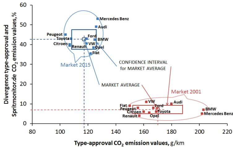
Fig. 2. Divergence type-approval and Spritmonitor.de CO<sub>2</sub> emission values as function of type-approval CO<sub>2</sub> emission values depending of the time
