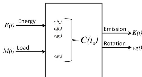
Fig. 3. Engine in a simplified system approach
