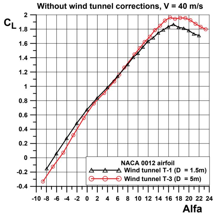
Fig. 7. Comparison of the  $C_L = f(\alpha)$  characteristic for the model of Tu-154M aircraft obtained in the low speed wind tunnels T-1 and T-3 without wind tunnel corrections
