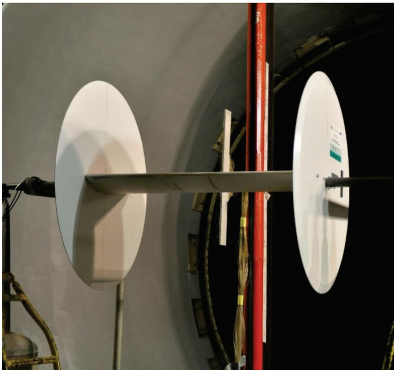
*Fig. 4. Model of the of the NACA 0012 airfoil in low speed wind tunnel T-3*
