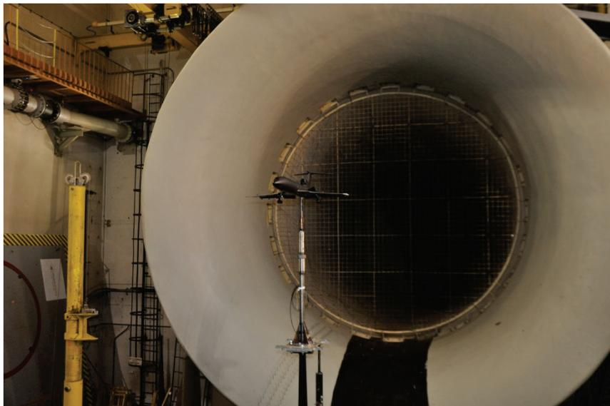
*Fig. 2. Model of the Tu-154M aircraft in low speed wind tunnel T-3*
