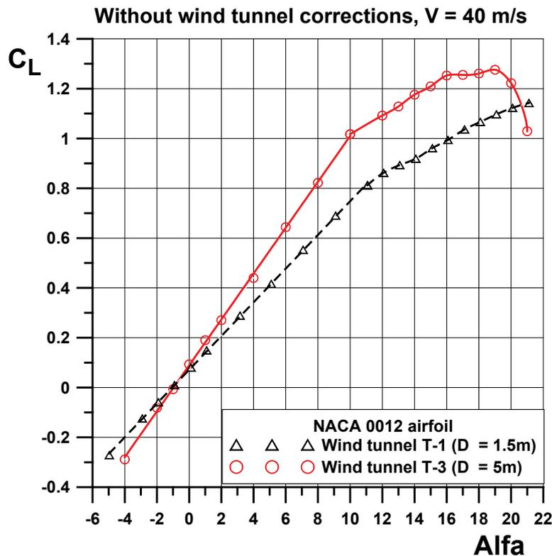
Fig. 5. Comparison of the  $C_L = f(\alpha)$  characteristic for the NACA 0012 airfoil obtained in the low speed wind tunnels T-1 and T-3 without wind tunnel corrections
