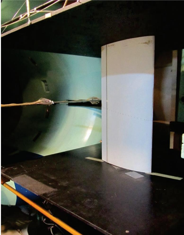
*Fig. 3. Model of the NACA 0012 airfoil in low speed wind tunnel T-1*
