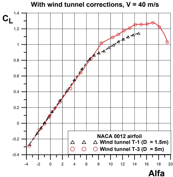
Fig. 6. Comparison of the  $C_L = f(\alpha)$  characteristic for the NACA 0012 airfoil obtained in the low speed wind tunnels T-1 and T-3 with wind tunnel corrections
