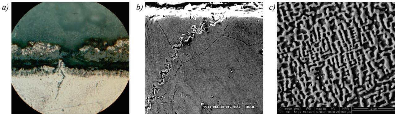
Fig. 6. An example of turbine blade overheating, a) heat-resistant coating delamination and rupture of its material b) SEM microstructure of a rupture with a trans-crystalline character –  $\times 450$  c) microstructure of the strengthening phase  $\gamma'$  in lamellar form –  $\times 5000$
