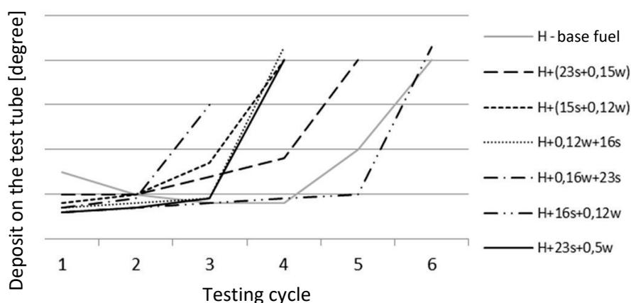
Fig. 1. Results of the test measuring the impact of additive dosage technology on fuel thermal stability (H – means hydro raffinate-based fuel, 15 s, 16 s, 23 s – content of additive s in mg/kg, 0.12 w, 0.15 w, 0.16 w, 0.5 w – content of additive in % (V/V), parenthesis means that the additives were added simultaneously, in the absence of the parenthesis – additives were introduces successively, a week apart) [2]
