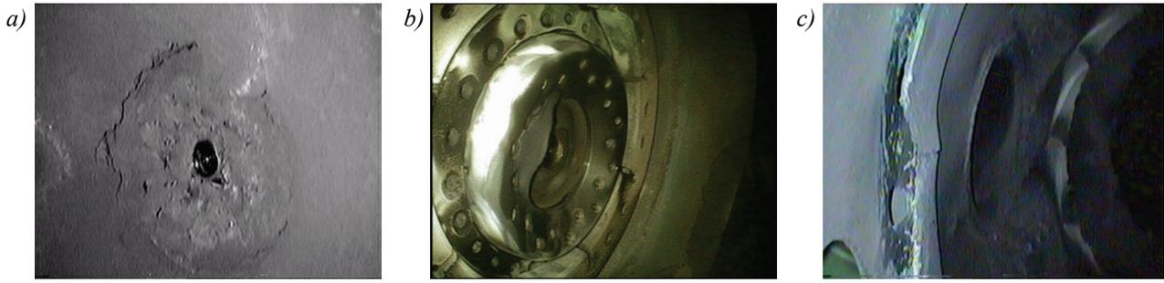
Fig. 2. Condition of fuel injectors and glow tube: a) carbon deposit along the perimeter, b) single-sided carbon deposit, c) burnout of glow tube
