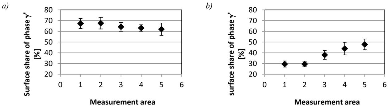
Fig. 7. The surface participation of strengthening phase  $\gamma'$  inside the edge of attack in individual blades: a) new blade, b) a blade after a significant period of operation (1 – blade surface)
