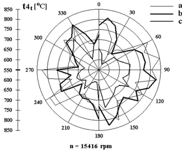
Fig. 3. Example results for measurements of the temperature field non-homogeneity within the working agent inside the jet nozzle of the K-16 engine: a – nearby the outer wall, b – in the middle of the gas duct radius c – nearby the inner wall [14]
