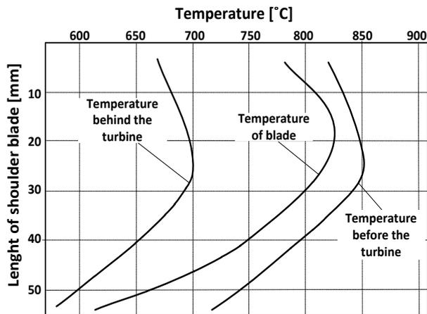
Fig. 4. Examples of flue gas temperature distribution radial profiles for an annular combustion chamber upstream and downstream of the turbine and their impact on the distribution of temperature in the blade material [9]
