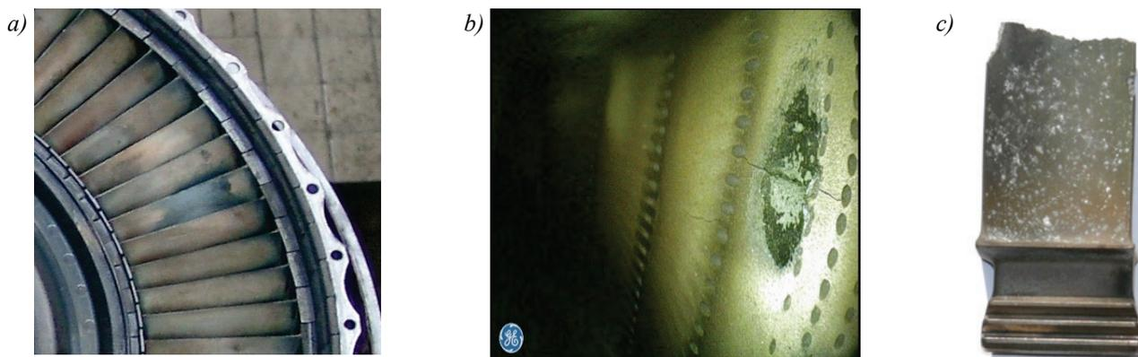
*Fig. 5. Forms of gas turbine damage: a) different colours on vanes surfaces exhibiting various overheating degree [13], b) nozzle apparatus vane with an overheating zone, c) rotor blade torn off due to burn-through*
