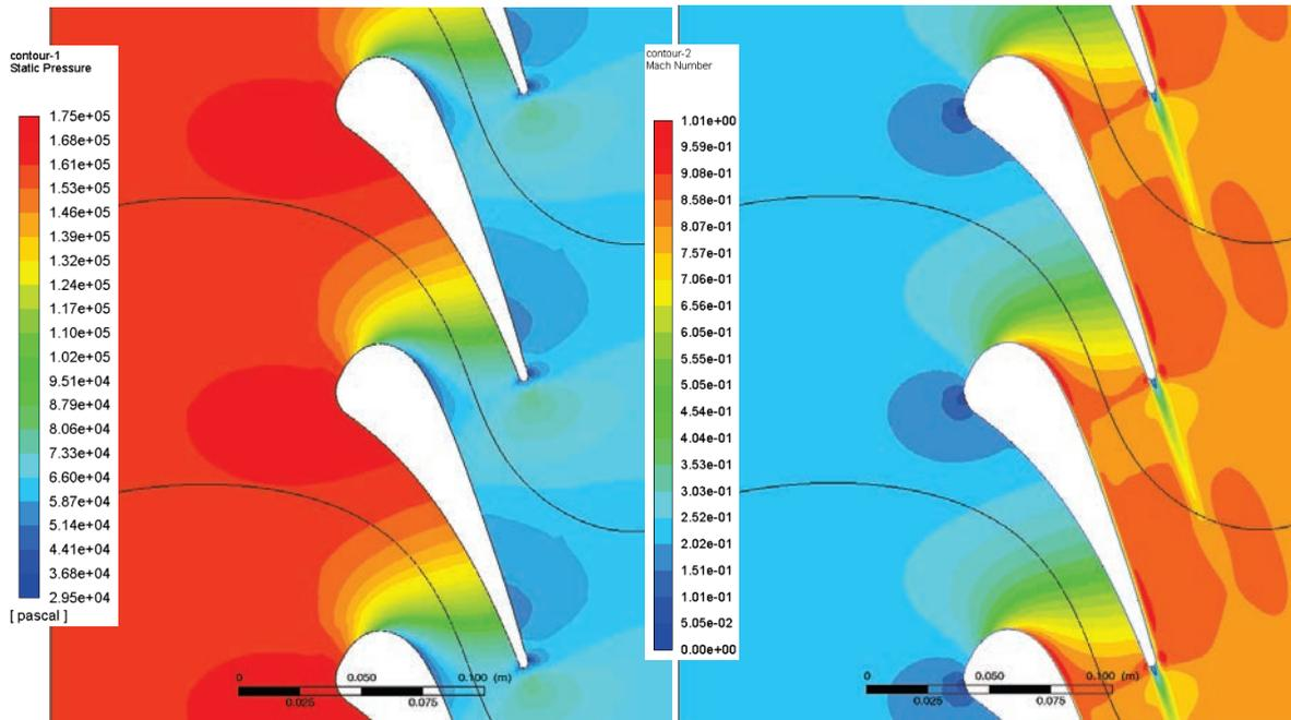
Fig. 3. Contours of Pressure and Mach number [Bugala, 2018]
