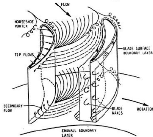
Fig. 1. Flow structure around a turbine cascade [7]
