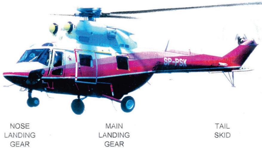
Fig. 1. W3 Helicopter. Source PZL-Świdnik
