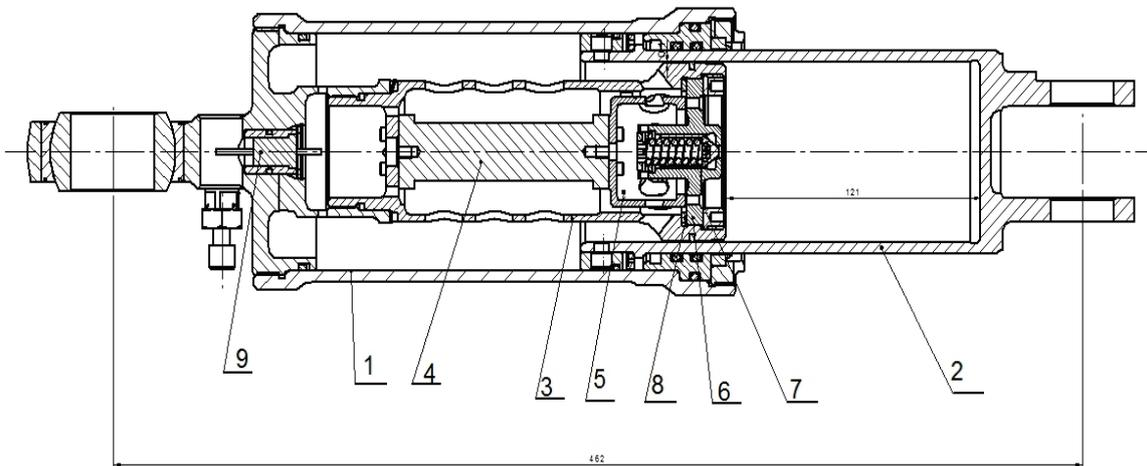
Fig. 2. ADLAND project piezo-valve solution: 1 – cylinder, 2 – piston, 3 – plunger, 4 – piezo-actuator, 5 – valve head, 6 – suppressing plate, 7 – nut, 8 – adjusting plate, 9 – culvert. Source ILOt
