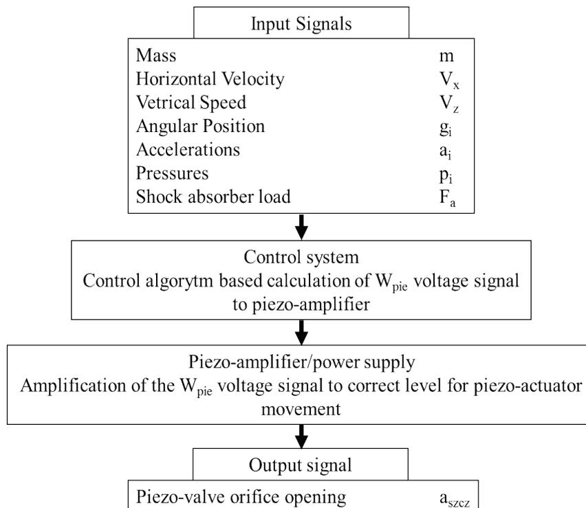
Fig. 3. Block diagram of the designed adaptive landing gear control system, source ILOT
