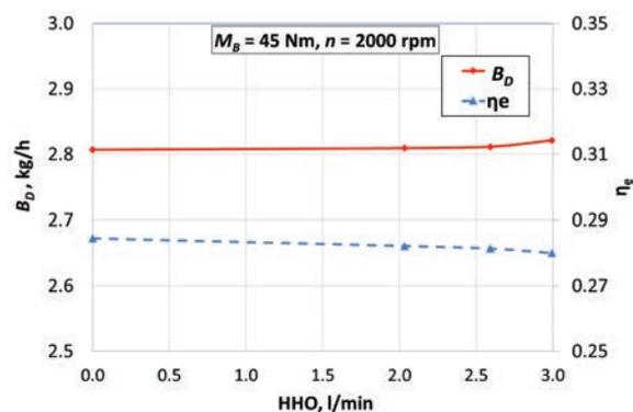
Fig. 5. HHO gas amount influence for hourly fuel consumption ( $B_D$ ) and engine efficiency ( $\eta_e$ )
