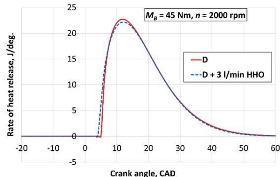
Fig. 9. Heat release in cylinder
