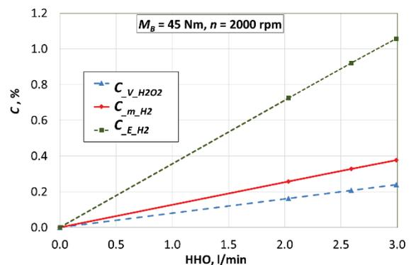
Fig. 3. The change of HHO gas volumetric concentration  $C_{v\_HHO}$ , the mass concentration of hydrogen  $C_{m\_H2}$ , and the concentration of hydrogen energy in the mixture of fuel  $C_{E\_H2}$
