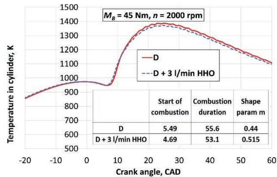
Fig. 7. Combustion process indicators and temperature in cylinder
