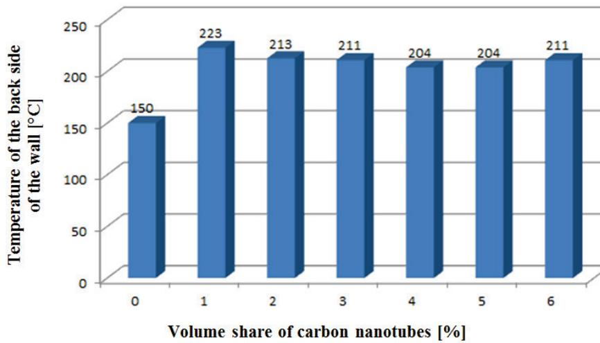
Fig. 5. Temperature of the rear surface of the insulating sample  $t_s$  [ $^{\circ}\text{C}$ ], depending on the volume share of carbon nanotubes after a period of 150 seconds of the exposition to a heat flux
