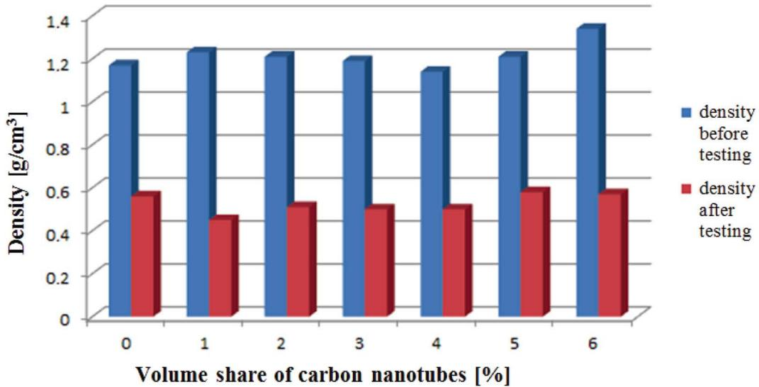
Fig. 2. Comparison of density of the composite samples before and after ablation testing
