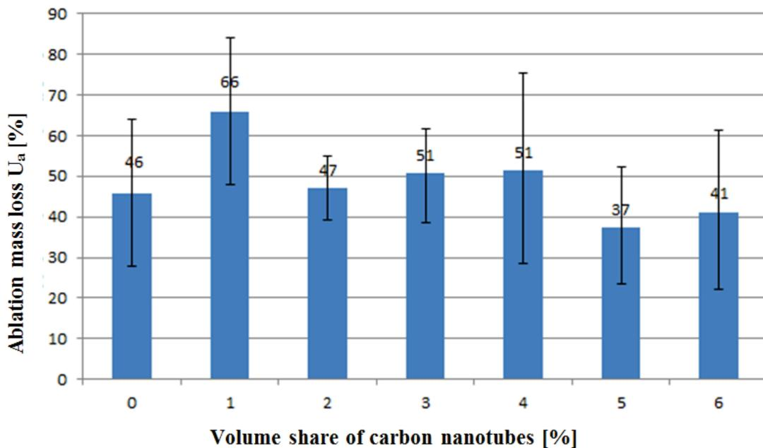
Fig. 3. Average relative ablation mass loss  $U_a$  [%], depending on the volume share of carbon nanotubes after a period of 150 seconds of the exposition to a heat flux
