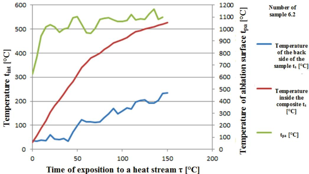
Fig. 7. Comparison of the temperature of ablation surface  $t_{pa}$  [°C], temperature inside the composite  $t_{int}$  [°C] and temperature on the rear surface of the wall  $t_s$  [°C] in sample no.2 of 6% volume share of carbon nanotubes after a period of 150 seconds of the exposition to a heat flux
