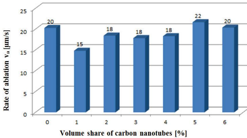
Fig. 4. Average ablation rate  $v_a$  [ $\mu\text{m}$ ], depending on the volume share of carbon nanotubes after a period of 150 seconds of the exposition to a heat flux
