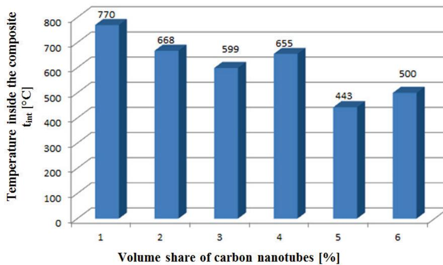
Fig. 2. Temperature inside the composite  $t_{\text{int}}$  [ $^{\circ}\text{C}$ ], depending on the volume share of carbon nanotubes after a period of 150 seconds of the exposition to a heat flux
