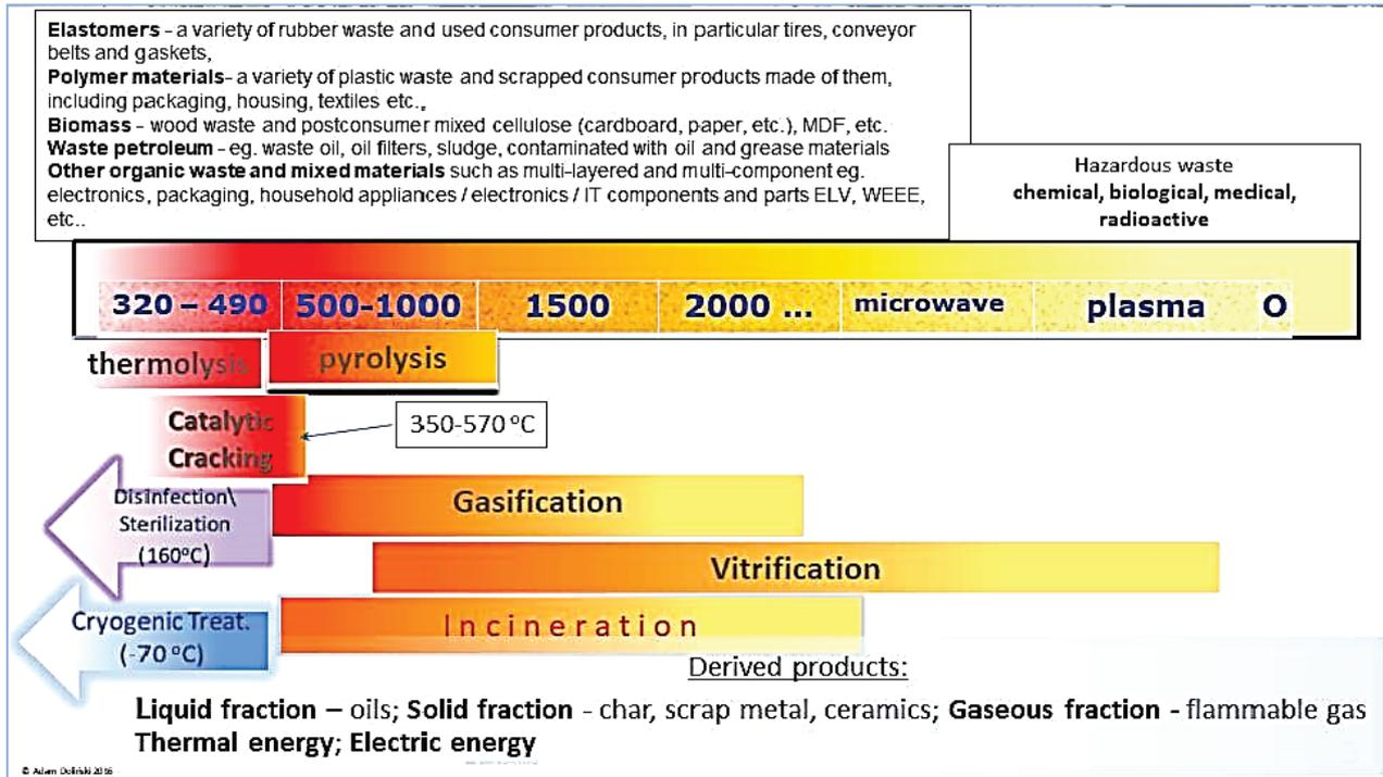
Fig. 5. Methods of thermal treatment of organic and mixed waste [2]
