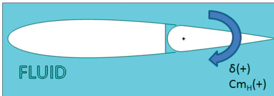
Fig. 1. Analysed representative cross section of an aircraft stabilizer, based on NACA0012 airfoil (with marked sign convention)
