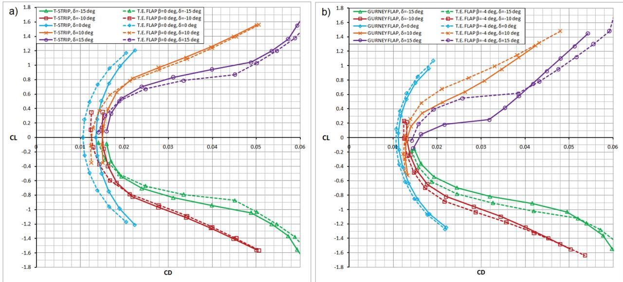
Fig. 5. CL(CD) characteristics for: a) T-strip and non-deflected TE flap; b) Gurney Flap and deflected TE flap
