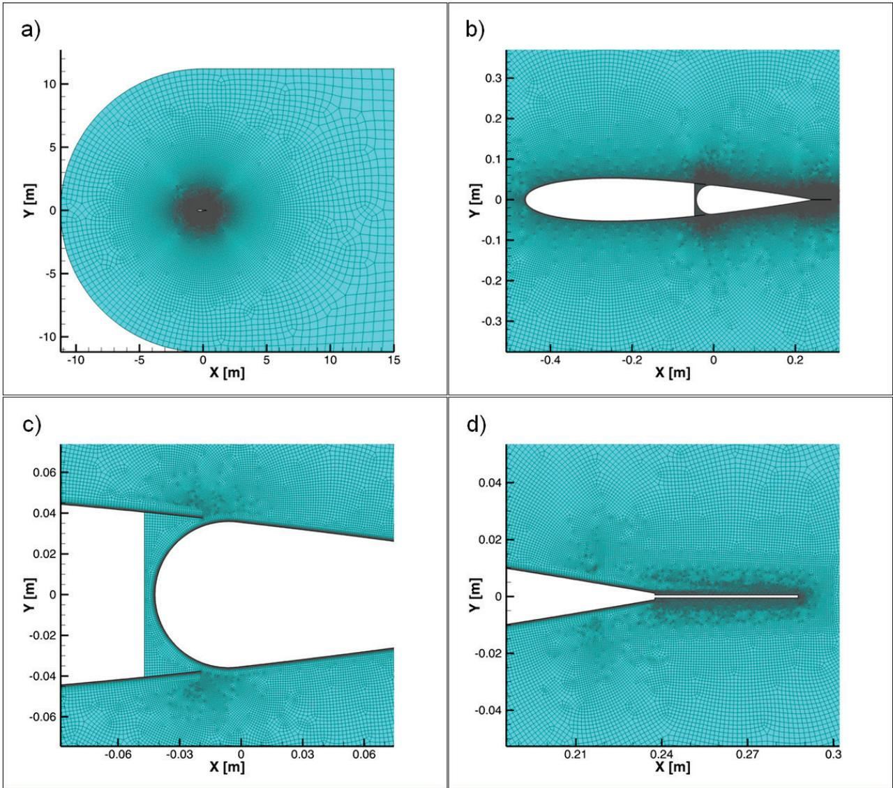
Fig. 3. Example meshes details around: a) the entire domain; b) the airfoil; c) the hinge gap; d) the non-deflected trailing edge flap
