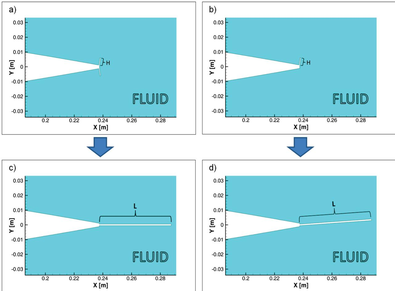
Fig. 2. Technical solutions analysed: a) Gurney Flap ( $H = 5 \text{ mm}$ ); b) T-strip ( $H = 5 \text{ mm}$ ); c) non-deflected trailing edge flap ( $L = 50 \text{ mm}$ ); d) deflected ( $-4$  degrees) trailing edge flap ( $L = 50 \text{ mm}$ )
