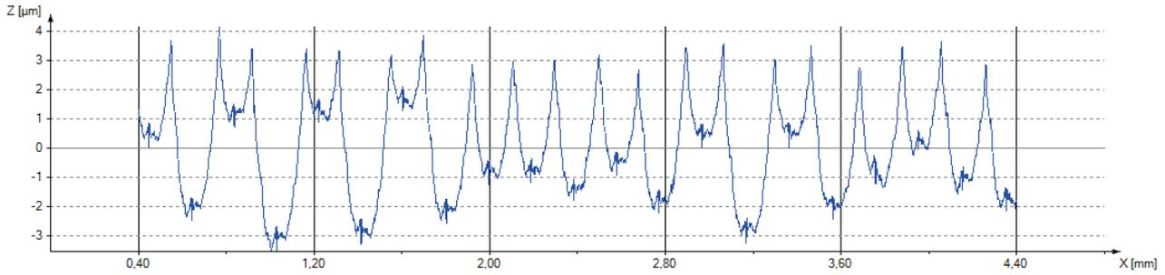
Fig. 1. Surface roughness profile made on the Hommel Etamic Waveline 20 profilometer
