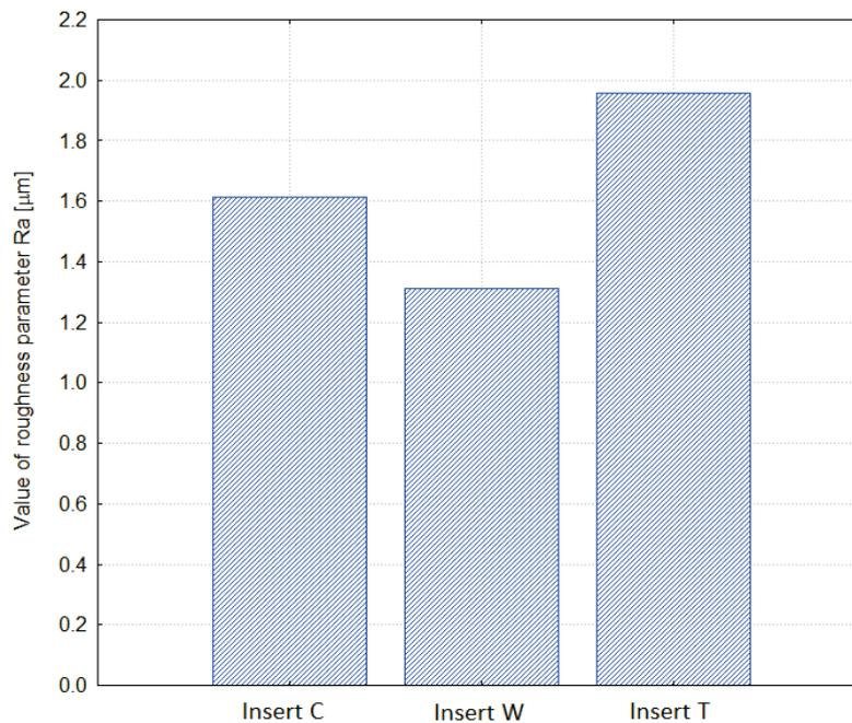
*Fig. 3. The graph of the second measurement results with the averaged values of the parameter  $R_a$*
