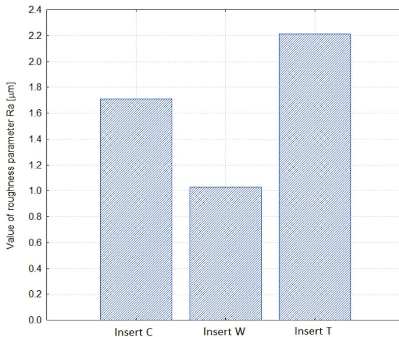
Fig. 4. The graph of the third measurement results with the averaged values of the parameter  $R_a$
