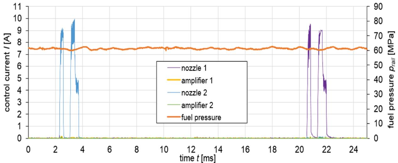
Fig. 4. Control current curves of CRIN4 injector for nozzle and amplifier valves and fuel pressure in the rail
