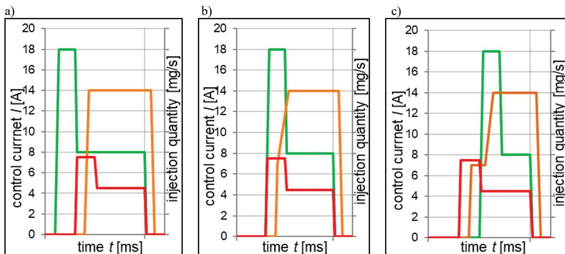
Fig. 2. Current curves for triggering nozzle valve (red), amplifier valve (green) and injection rate (orange) for square type injection (a), ramp (b) and boot (c)
