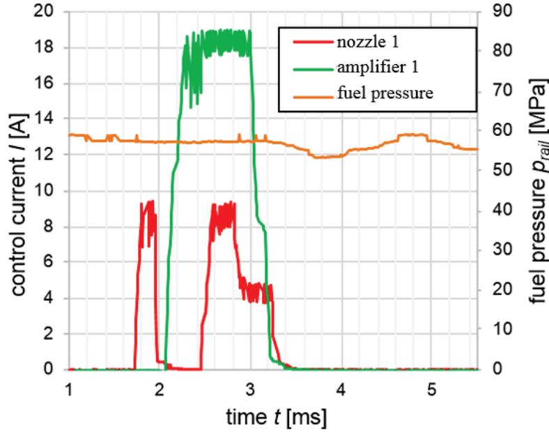
Fig. 6. Control current curve for square type injection and fuel pressure for  $n_s = 1200$  rpm,  $M_o = 250$  Nm
