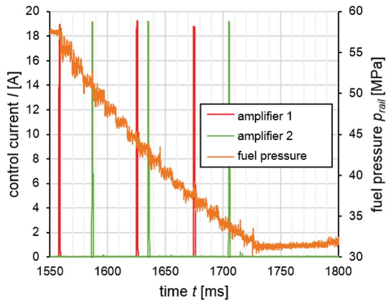
*Fig. 9. Fuel pressure regulation caused by amplifier valves triggering,  $n_s = 2200 \text{ rpm}$ ,  $M_o = 0 \text{ Nm}$*
