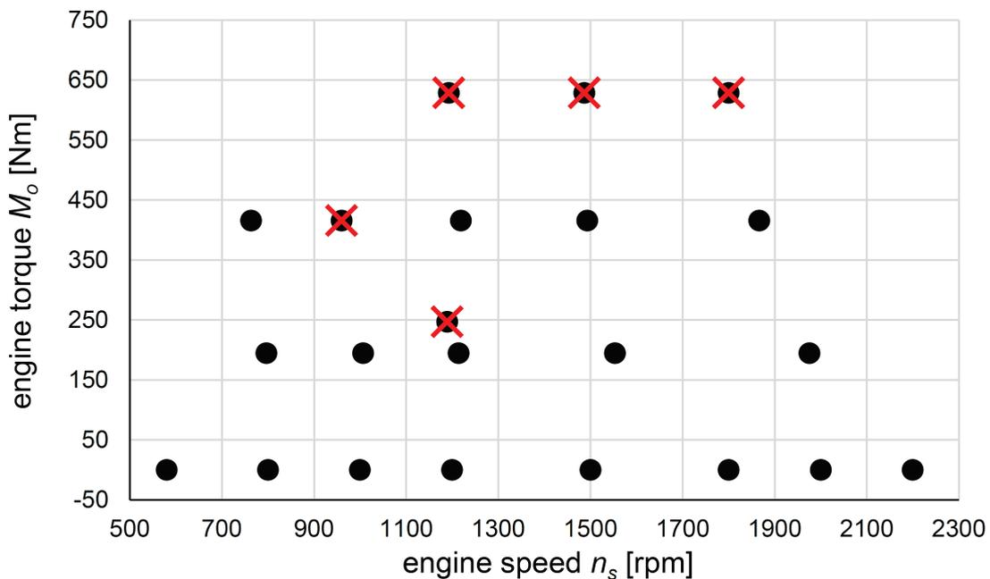
Fig. 5. Measuring points determined by engine speed and torque
