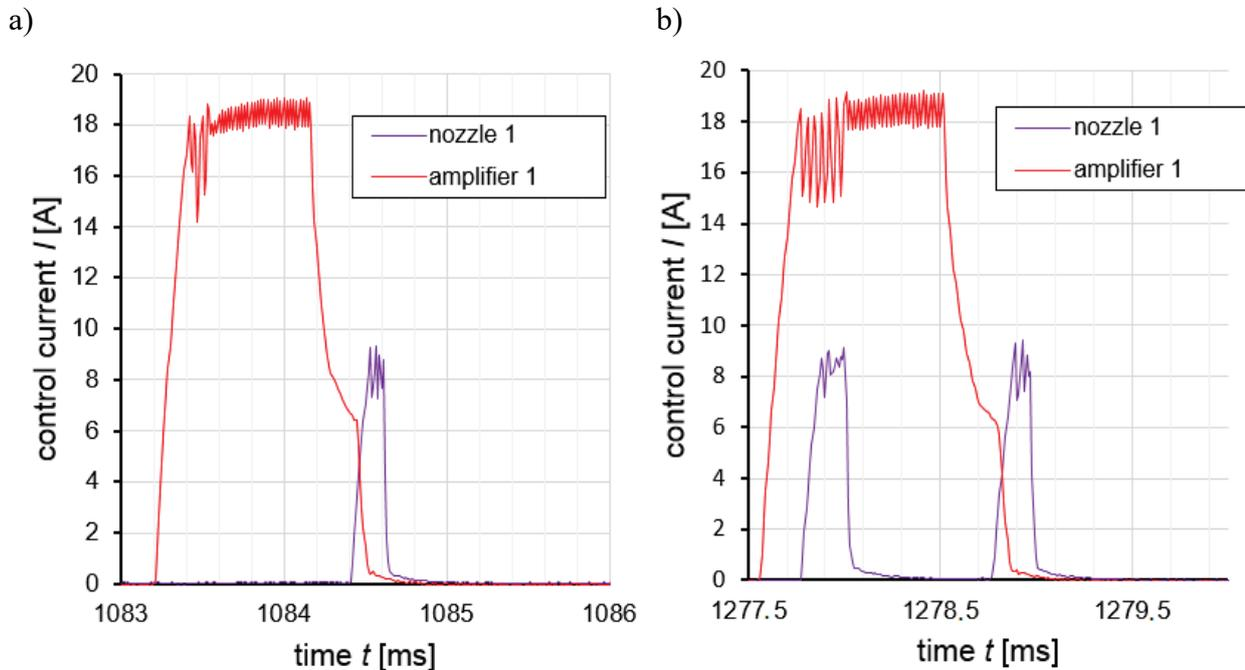
Fig. 10. Short nozzle valve activation during fuel pressure regulation by amplifiers,  $n_s = 1200$  rpm
