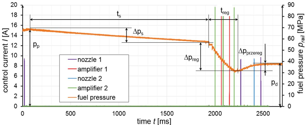
Fig. 8. Control current curves and fuel pressure during fuel pressure reduction performed by amplifiers  $n_s = 1800$  rpm;  $M_o = 0$  Nm
