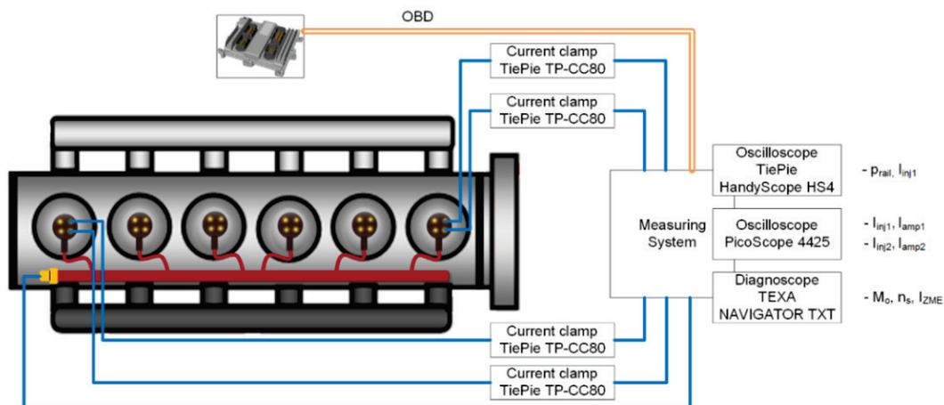
Fig. 3. Measuring system for acquisition control signals and fuel pressure signal of CRIN4 common rail with CRIN4 injectors applied in OM 471.9 engine
