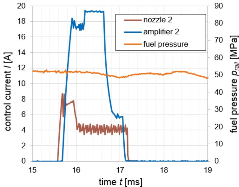
Fig. 7. Control current curve for boot type injection and fuel pressure for  $n_s = 1000$  rpm,  $M_o = 420$  Nm
