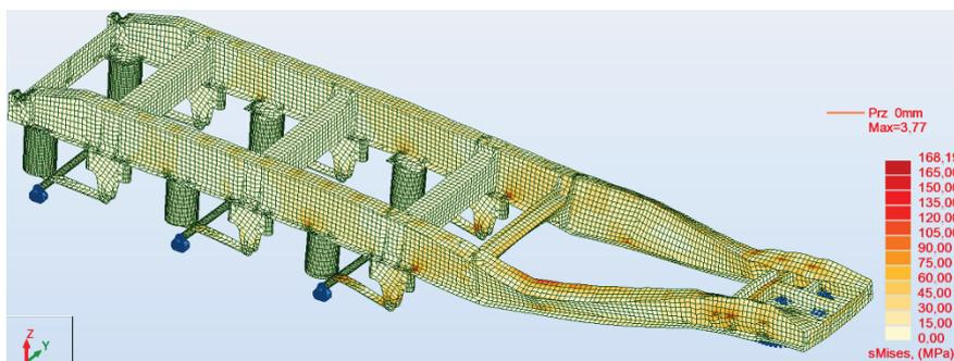
Fig. 4. Deformation of the frame at the old crossbar position
