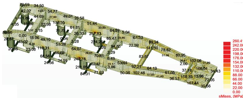
Fig. 10. Stress distribution in the frame during braking
