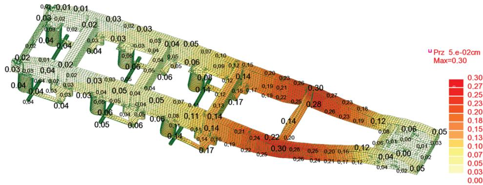
Fig. 11. Frame deformation during braking
