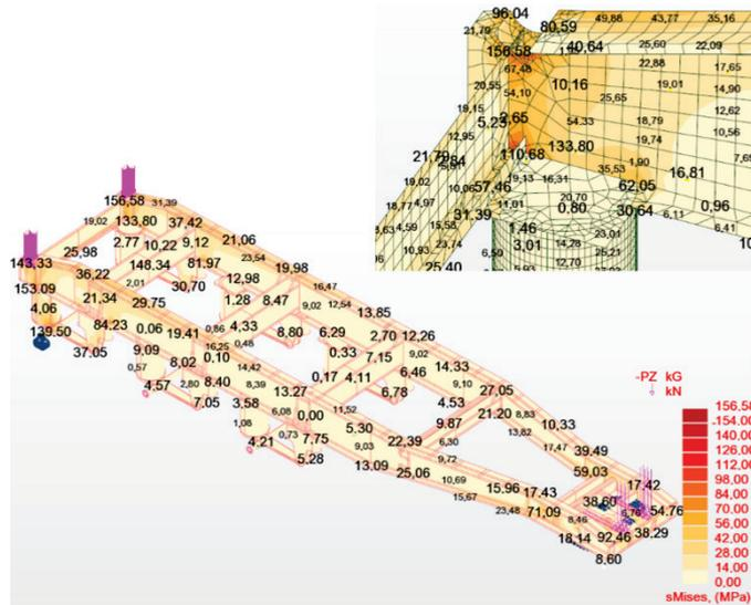
Fig. 8. Stress distribution in the frame during tipping
