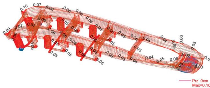
Fig. 9. Frame deformation during tipping
