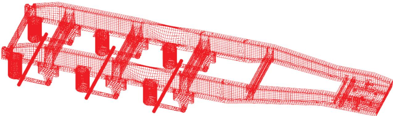
Fig. 6. Loss of strings stability of the frame
