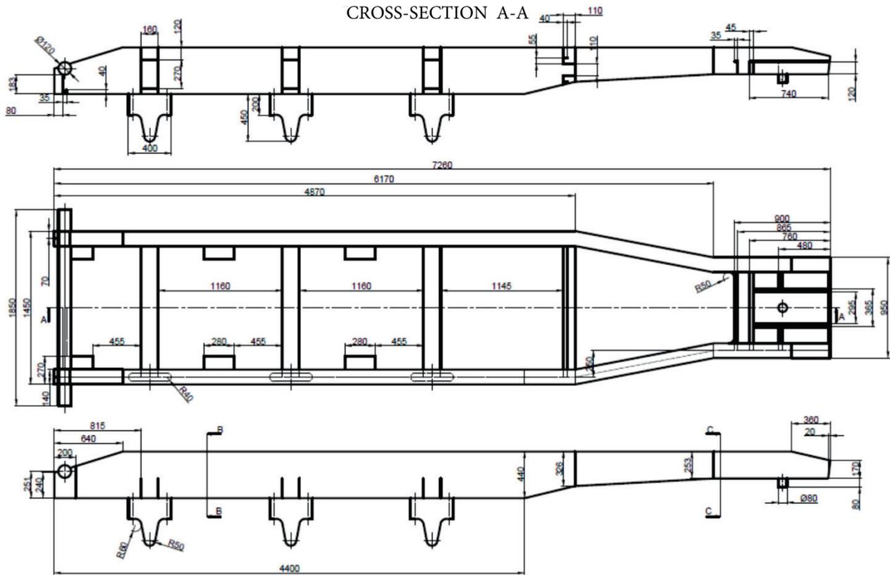
Fig. 1. Scheme of a semi-trailer frame
