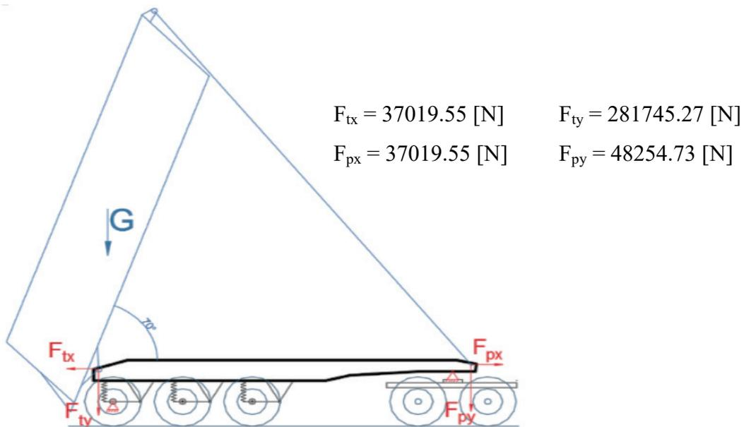
Fig. 7. Computational scheme for the tipping of the load box
