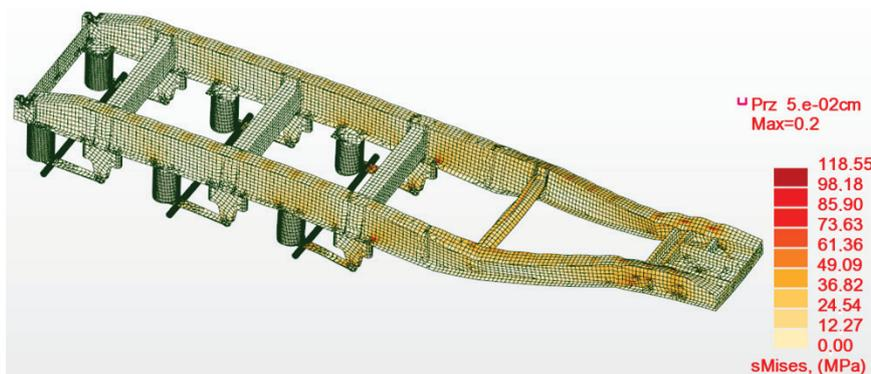
Fig. 5. Deformation of the frame at the new crossbar position
