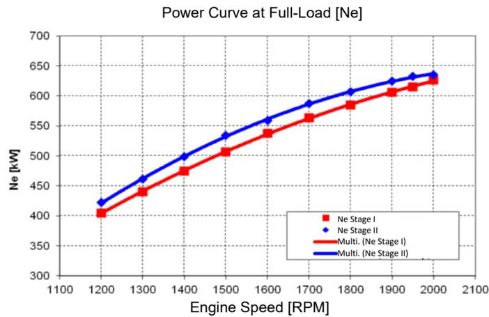
Fig. 5. Comparison of the S12-U power with pistons made of novel composite alloy and PA alloy forged piston
