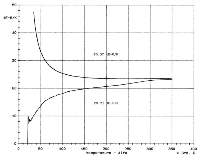
Fig. 2. Thermal expansion coefficient as a function of temperature from ambient temperature to 350°C during heating and cooling of the forged piston PA alloy
