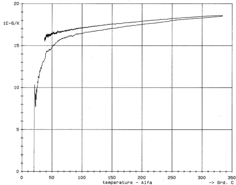
Fig. 1. Thermal expansion coefficient as a function of temperature from ambient temperature to 350°C during heating and cooling of the novel composite alloy
