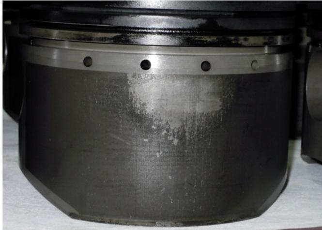
*Fig. 11. Friction markers formed on a piston surface which appear during engine operation*
