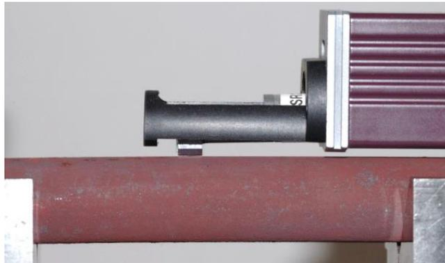
Fig. 2. The Mitutoyo profilograph Surface Roughness Tester SJ-301 type, according to [author's own archives]
