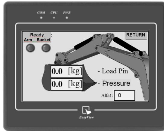
Fig. 5. HMI screen with function of weighing system
