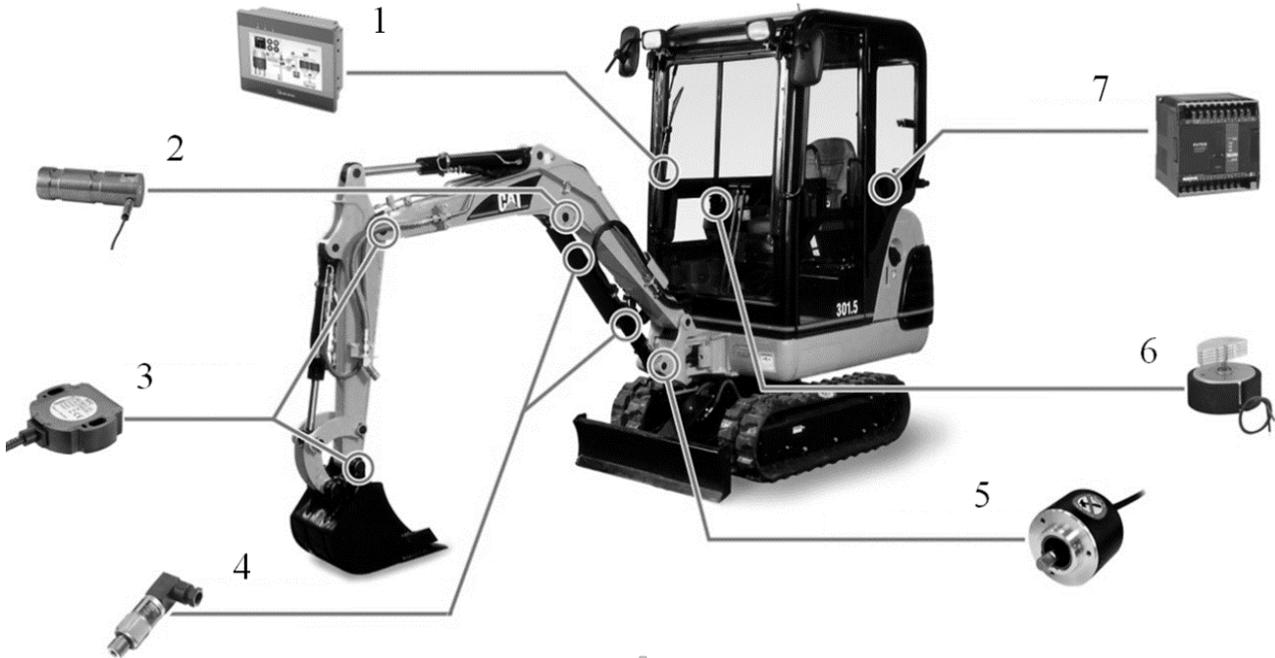
Fig. 4. Dynamic weighing system mounted on CAT 301.5
