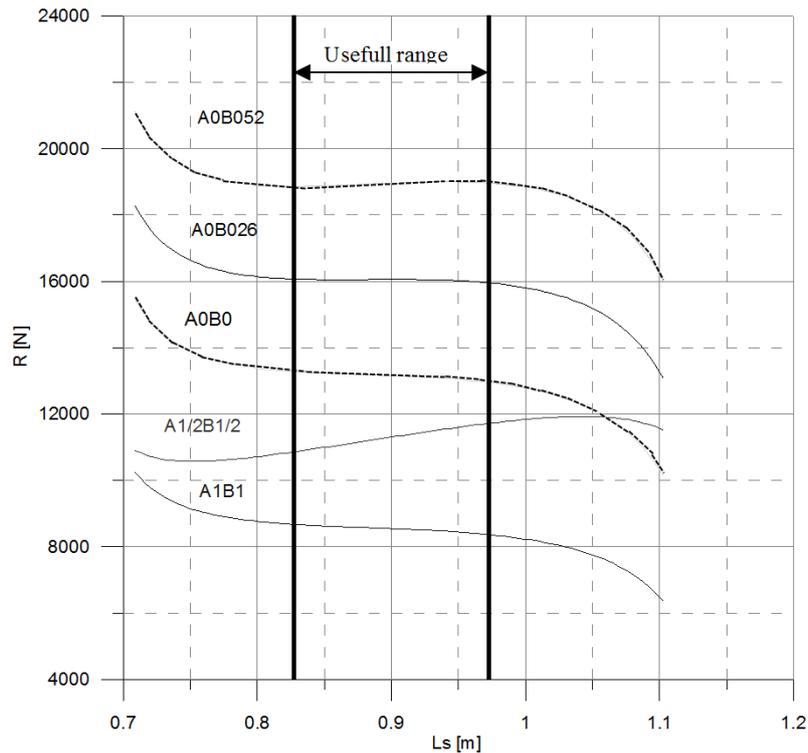
Fig. 3. Force  $R$  in function of boom cylinder length
