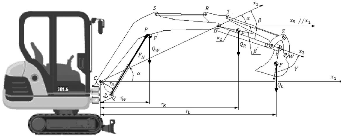
Fig. 1. Examples of excavator's geometric parameters used to determination mass of payload
