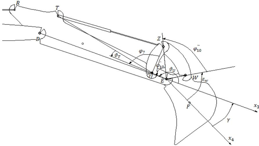
Fig. 2. Geometric parameters of arm and bucket mechanism
