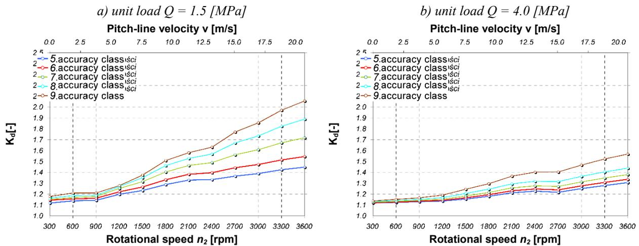
Fig. 4. Influence of quality class and rotational speed of wheel in toothed gear on values of dynamic coefficient  $K_d$ ; positive value of total periodic deviation [10]
