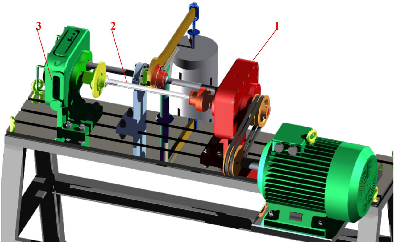
Fig. 1. Test stand with the gears operating in the circulating power system (FZG) [10]
