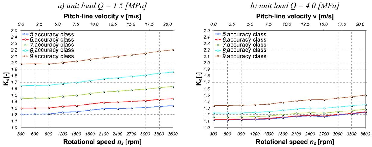
Fig. 5. Influence of quality class and rotational speed of wheel in toothed gear on values of dynamic coefficient  $K_d$ ; toothed gear without tip and root relief [10]
