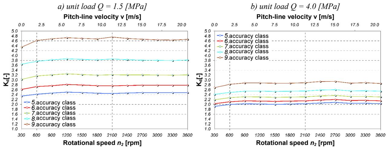
Fig. 3. Influence of quality class and rotational speed of wheel in toothed gear on values of dynamic coefficient  $K_d$ ; negative value of total periodic deviation [10]
