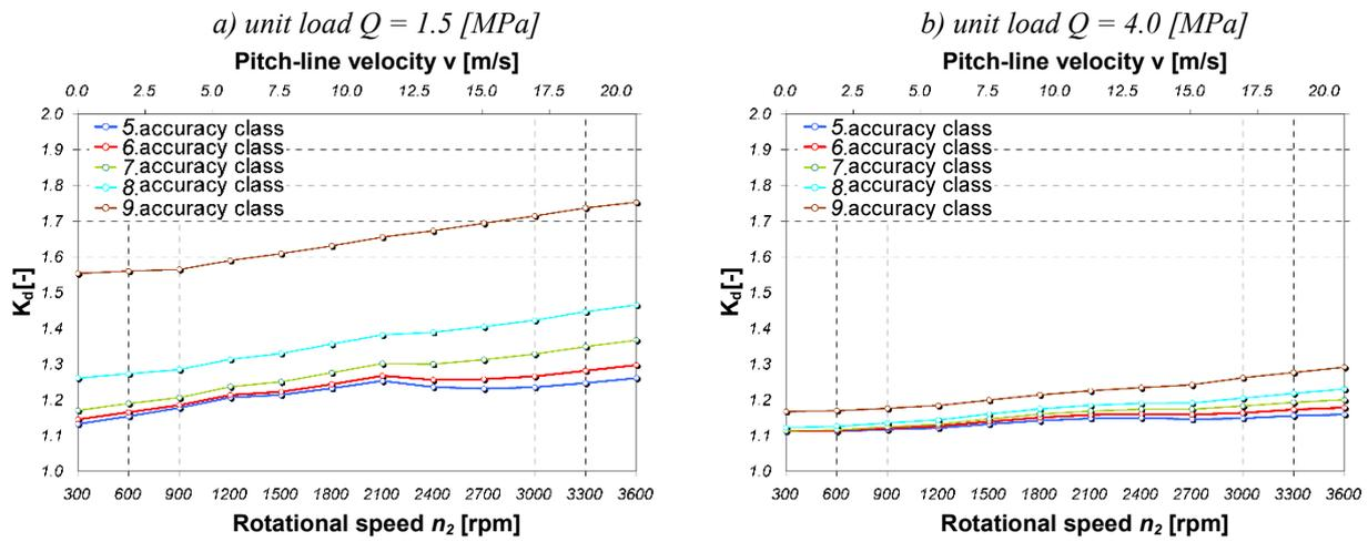
Fig. 6. Influence of quality class and rotational speed of wheel in toothed gear on values of dynamic coefficient  $K_d$ ; toothed gear with tip and root relief – type A [10]
