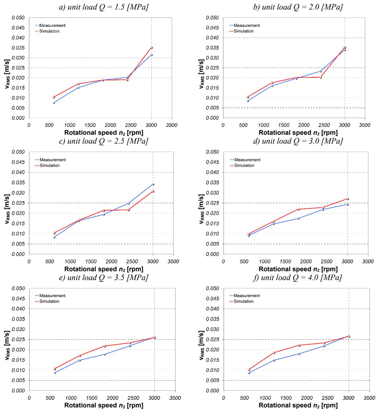
Fig. 2. Comparisons of the RMS values of the transverse vibration velocity of the gear wheel shaft, measured at test stand with the gears operating in the circulating power system and obtained from the model [10]
