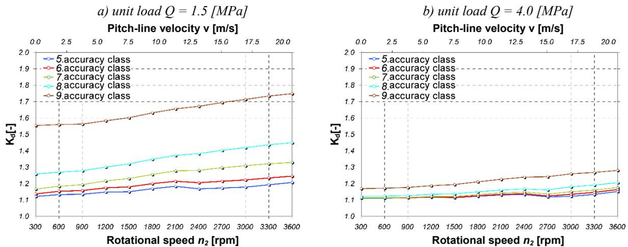
Fig. 7. Influence of quality class and rotational speed of wheel in toothed gear on values of dynamic coefficient  $K_d$ ; toothed gear with tip and root relief – type B (according to Maag) [10]
