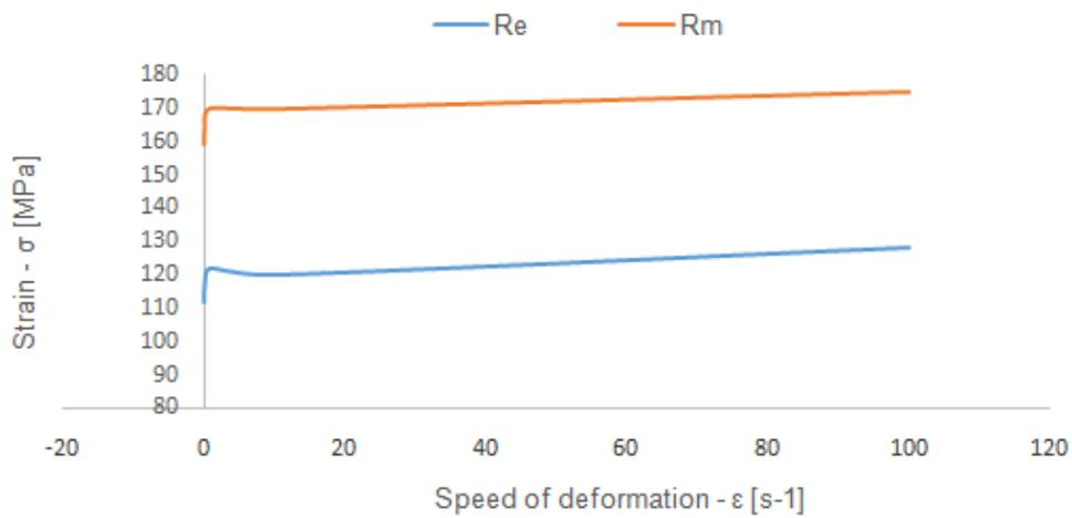
Fig. 7. Effect of deformation rate on yield strength and aluminum alloy strength 6060 T66
