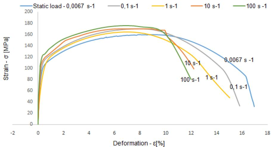
Fig. 5. Dependency graphs  $\sigma = f(\epsilon)$  with static and dynamic strain rates
