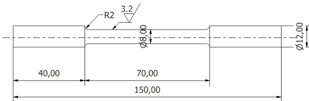
Fig. 3. Geometry of samples subjected to static and dynamic tensile testing according to PN-EN ISO 6892-1 2010P
