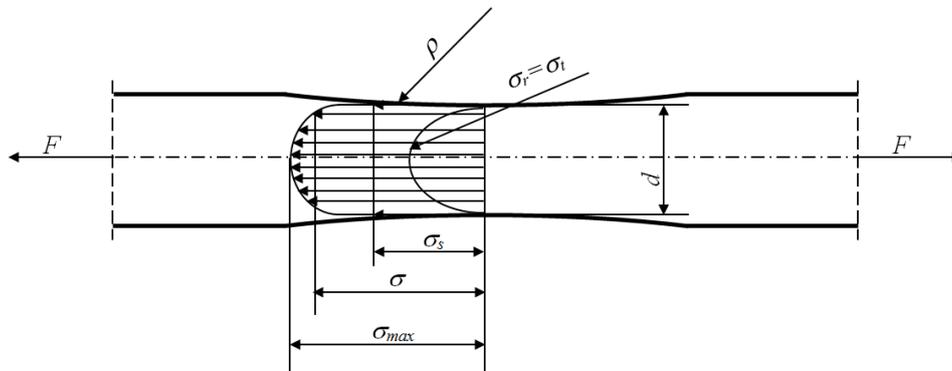
Fig. 2. Scheme of stress distribution in the neck of the stretched sample [3, 5]
