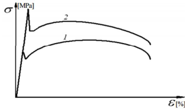
Fig. 1. The dependence graphs  $\sigma = f(\epsilon)$  with the velocity of static (1) and dynamic (2) [5]
