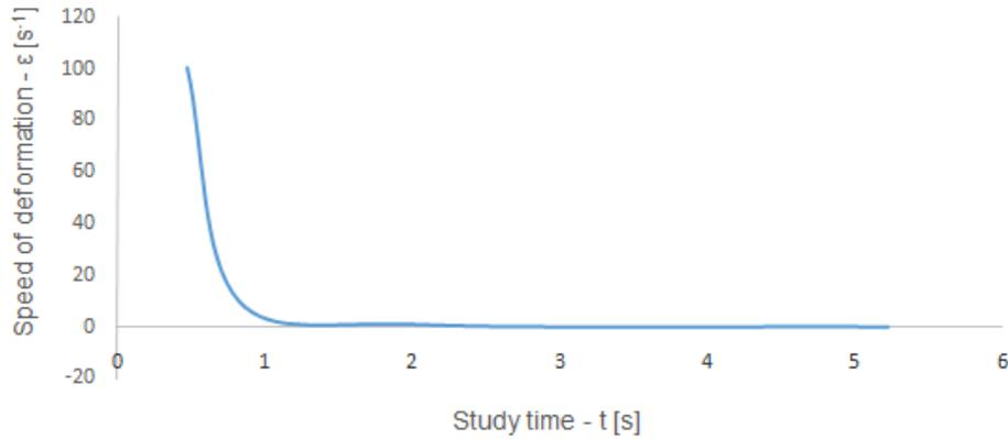
Fig. 6. Dependence of strain rate from test time for dynamic tensile test of alloy 6060 T66, based on data obtained after the test
