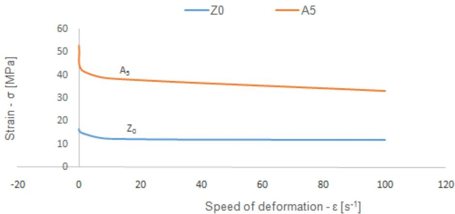
Fig. 8. The effect of the deformation rate on the total elongation (A5) and the constriction (Z0) of the aluminum alloy 6060 T66
