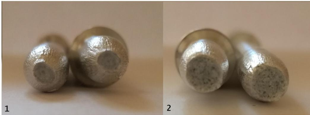
Fig. 9. Breakthroughs of selected samples: 1) after static stretching test, 2) after dynamic stretching with velocity  $100\text{ s}^{-1}$
