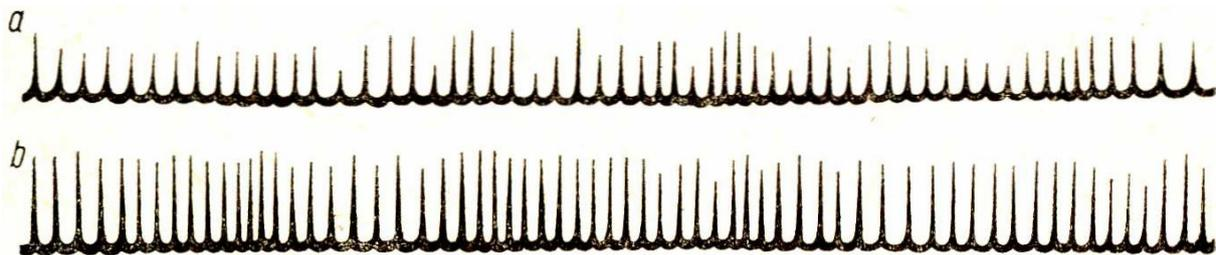
Fig. 4. Concentrated indicator diagrams: a – idle, b – high engine load [5]
