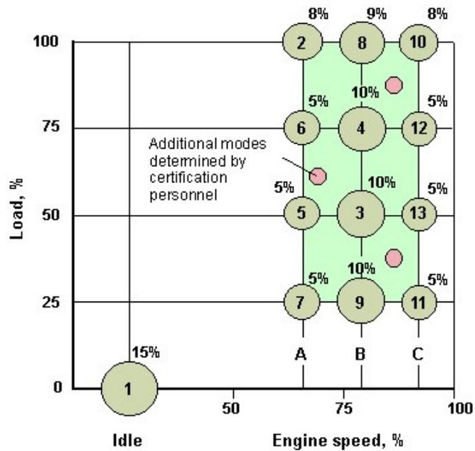
Fig. 6. The ESC characteristic diagram [3]
