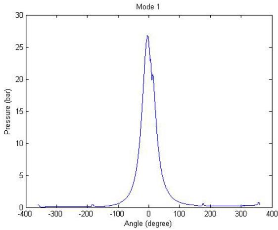
*Fig. 8. The indicator diagram*
