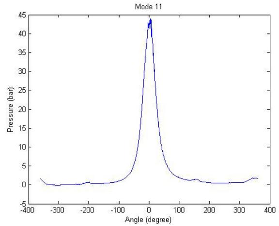
*Fig. 11. The indicator diagram*
