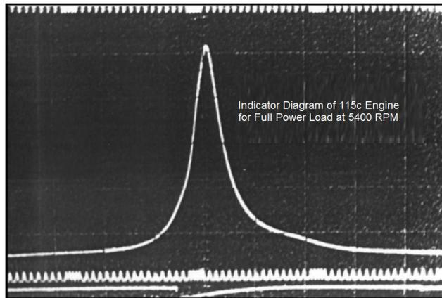
Fig. 3. Open indicator diagram [4]
