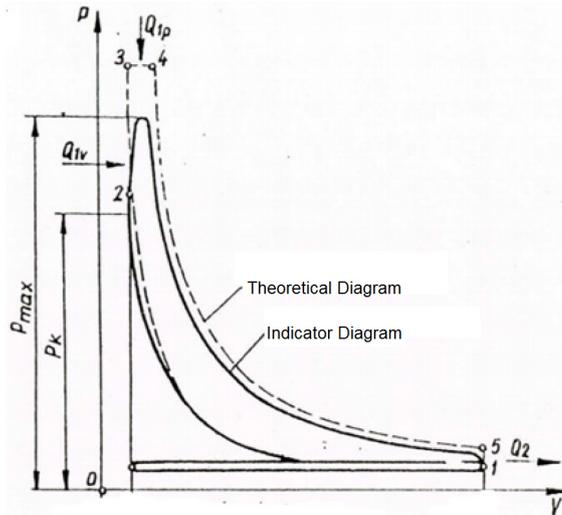
Fig. 1. Comparison of the theoretical and indicated diagrams [2]
