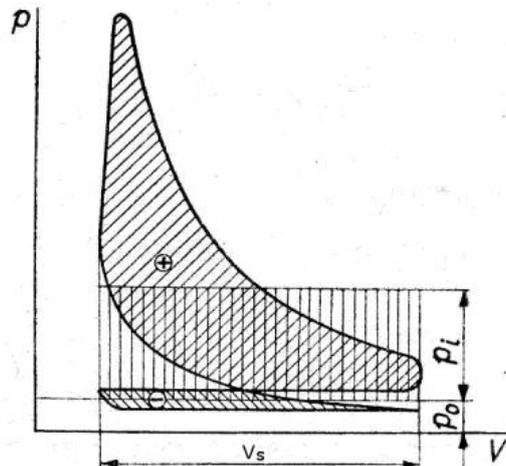
Fig. 2. Mean indicated pressure in Diesel engine [4]
