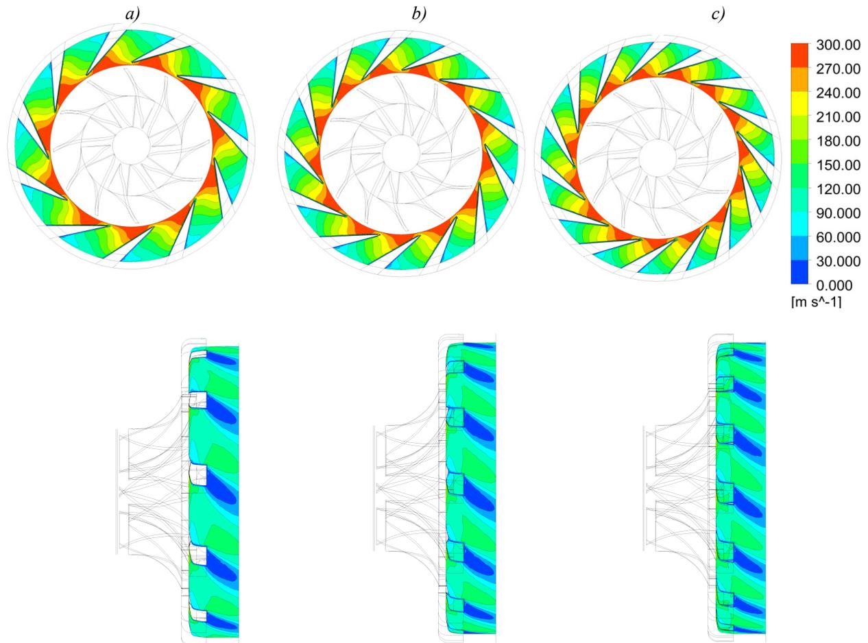
*Fig. 6. Velocity distribution in diffuser area a) 11 blades, b) 13 blades, c) 15 blades*
