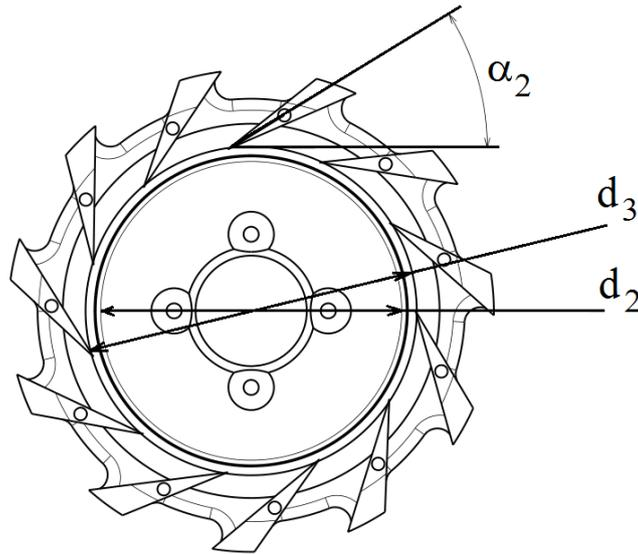
Fig. 1. Micro turbo jet engine diffuser characteristic dimensions
