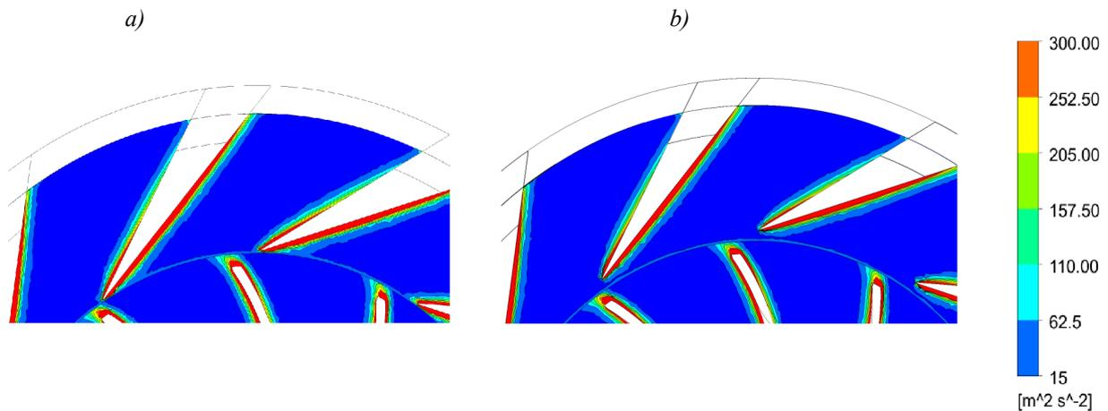
Fig. 3. Vanless diffuser space effect on turbulence intensity, a) value of  $x_3$  coefficient 1.0475, b) value of  $x_3$  coefficient 1.0745
