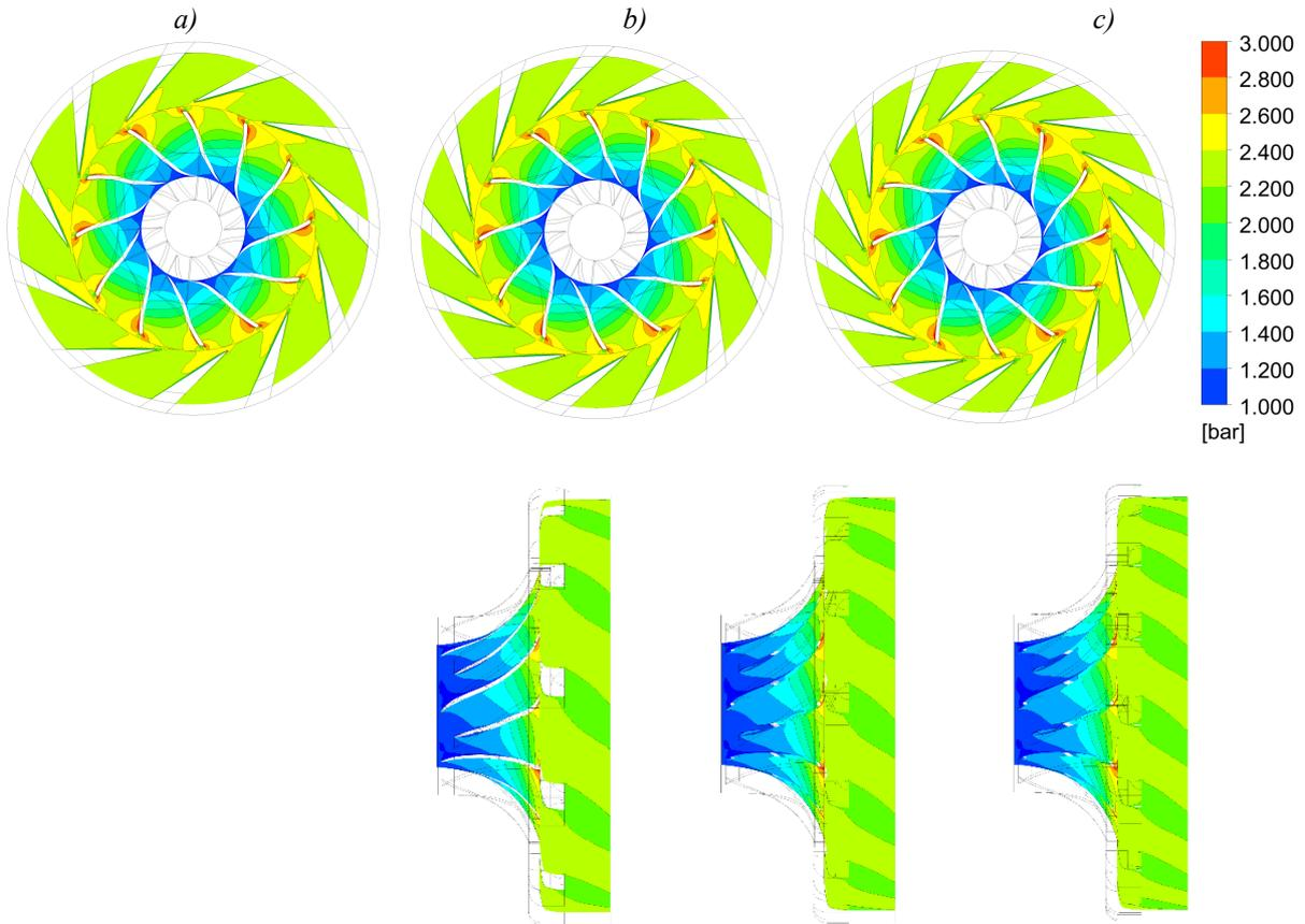
Fig. 5. Total pressure distribution a) 11 blades, b) 13 blades, c) 15 blades
