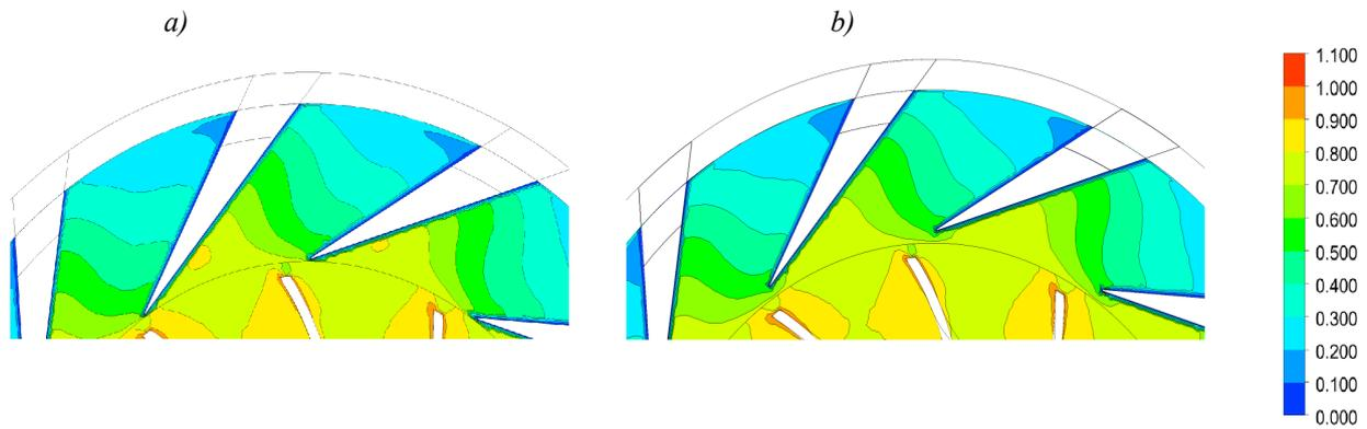
Fig. 2. Vanless diffuser space effect on a Mach number. a) Value of  $x_3$  coefficient 1.0475, b) value of  $x_3$  coefficient 1.0745
