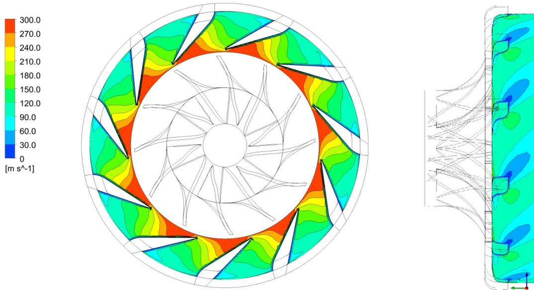
*Fig. 9. Velocity profile distribution in modified design*
