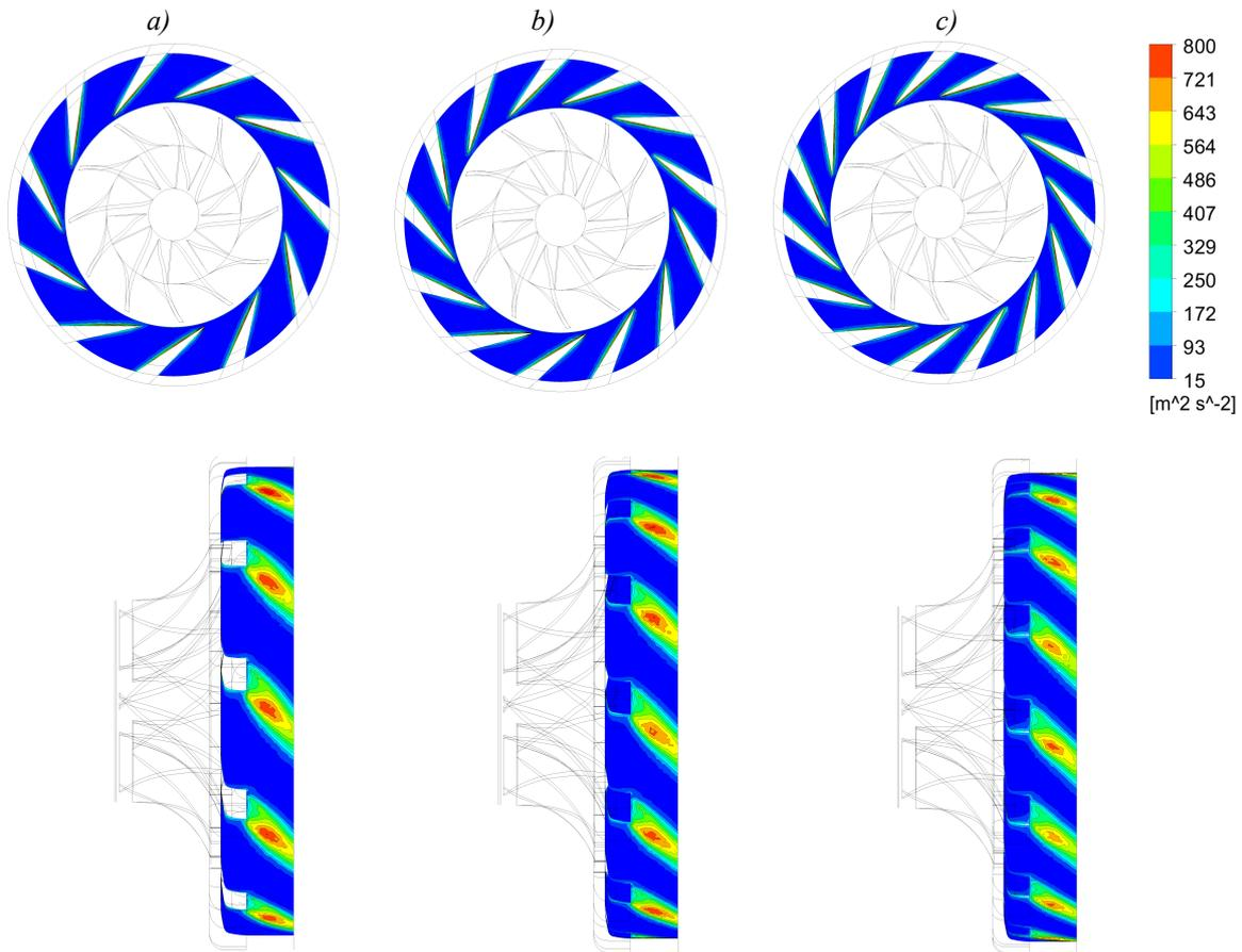
Fig. 7. Turbulence distribution in diffuser area a) 11 blades, b) 13 blades, c) 15 blades
