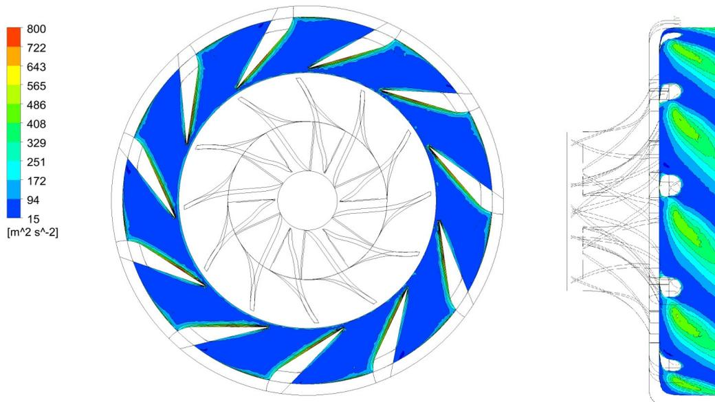
*Fig. 10. Modified design – turbulence intensity.*
