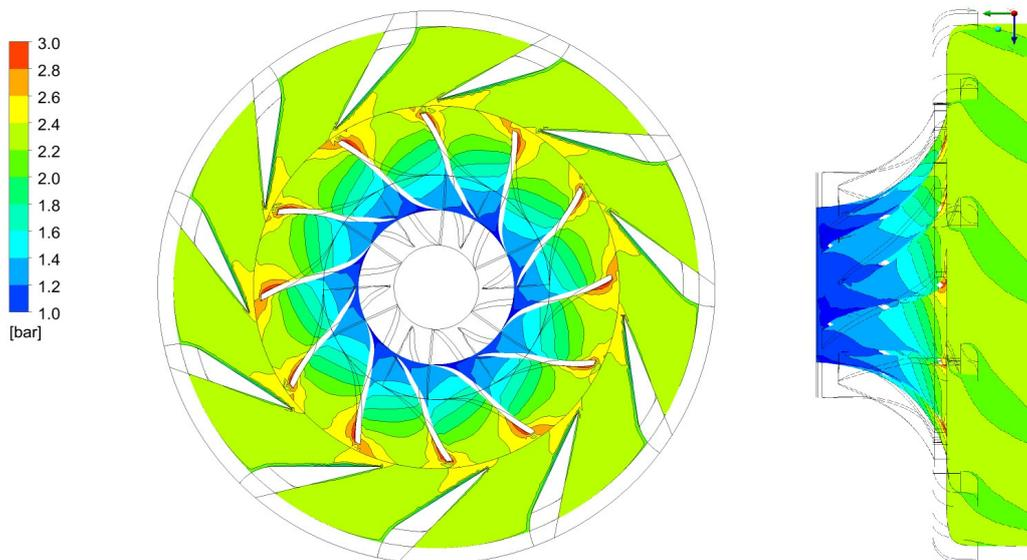
Fig. 8. Total pressure distribution in modified design
