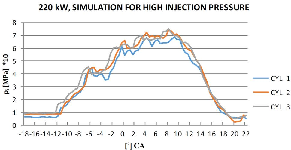
Fig. 9. Course of injection pressure curves at a specified load of 220 kW and simulated injector failure on cylinder number two
