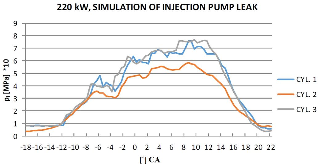
Fig. 10. Course of injection pressure curves at a specified load of 220 kW and simulated leakage failure on injection pump on cylinder number two
