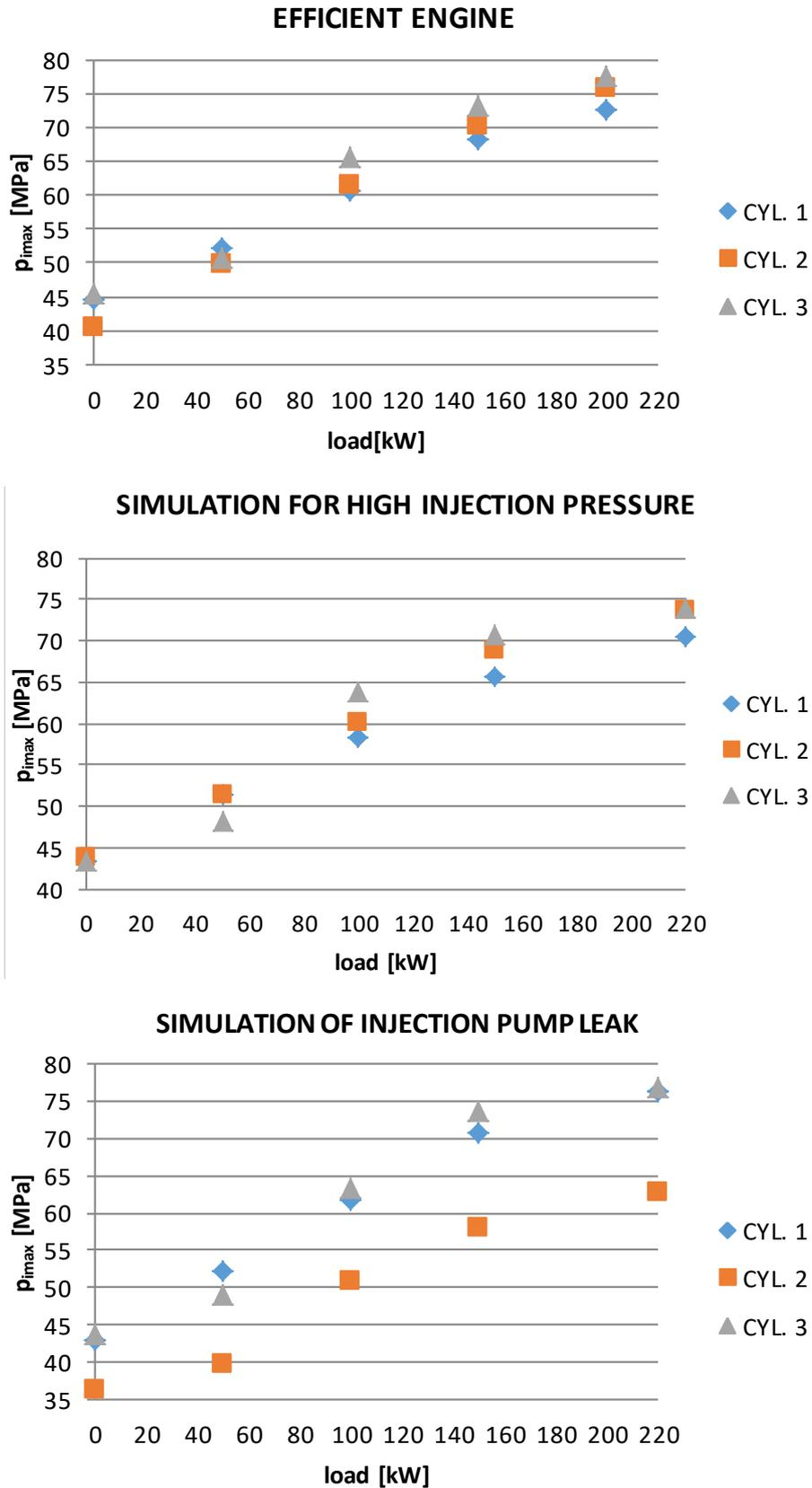
Fig. 7. The injection pressure sequence as a function of the load for the three cylinders
