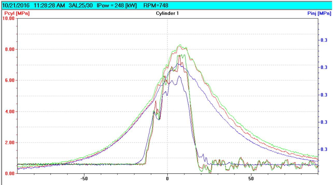
Fig. 6. Graphical representation of fuel injection pressure and combustion chamber pressure for simulated leakage failure on an injection pump at a specified load of 220 kW
