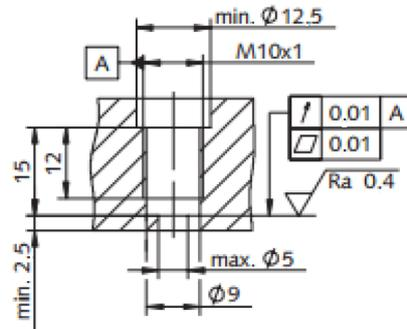
Fig. 4. How to make a hole fixing the transducer directly on the high-pressure conduit
