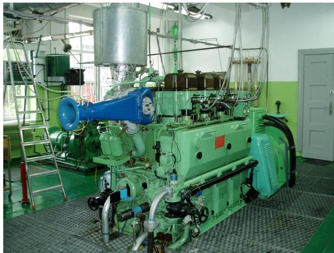
*Fig. 1. Photo of the piston engine SULZER 3AL25/30*
