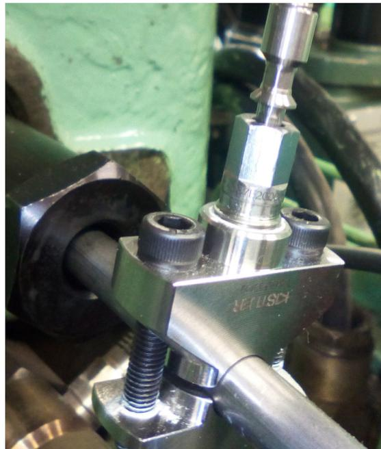
Fig. 5. Mounting the pressure sensor with the adapter
