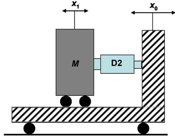
Fig. 5. Schematic of a vibration isolation system with variable friction device D2
