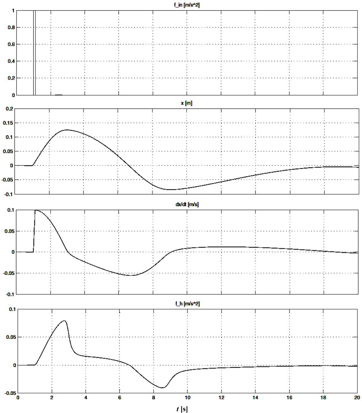
Fig. 6. The dynamic behaviour of device D2 used as a shock isolation system
