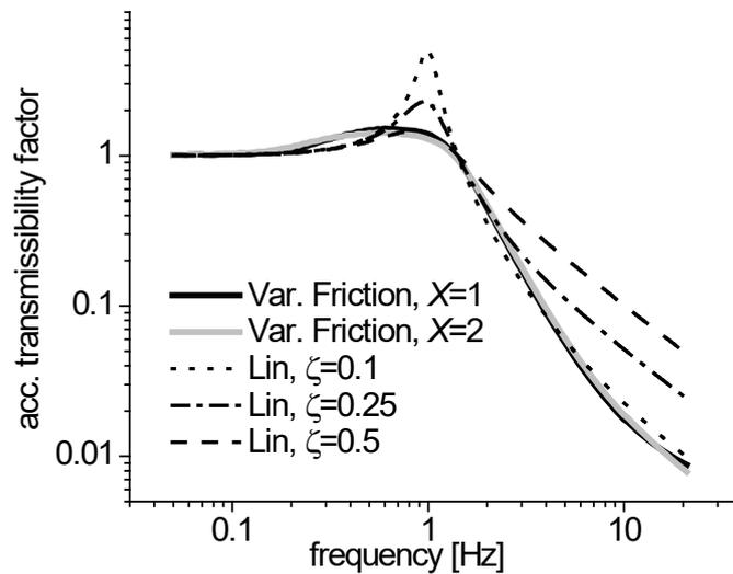
Fig. 7. Transmissibility factors of vibrations isolation systems with variable friction and of linear system
