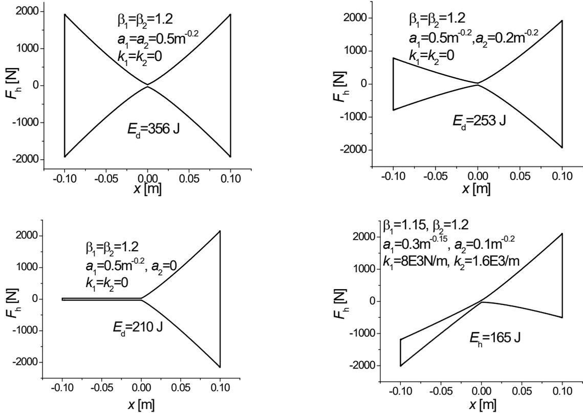
Fig. 3. Examples of hysteresis characteristics developed by the proposed device with variable friction
