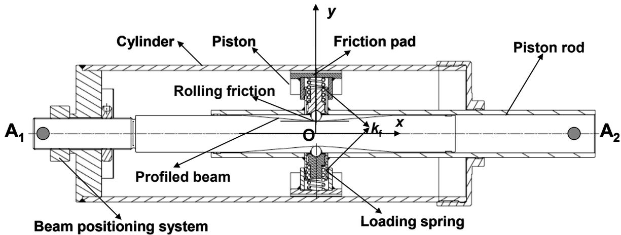
Fig. 1. The schematic of proposed damping system with variable friction D1
