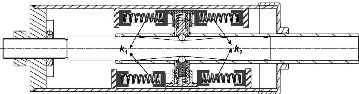
Fig. 2. The schematic of proposed system with variable friction for isolation of shock and vibrations D2
