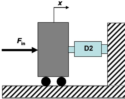
Fig. 4. Schematic of a shock isolation system with variable friction device D2
