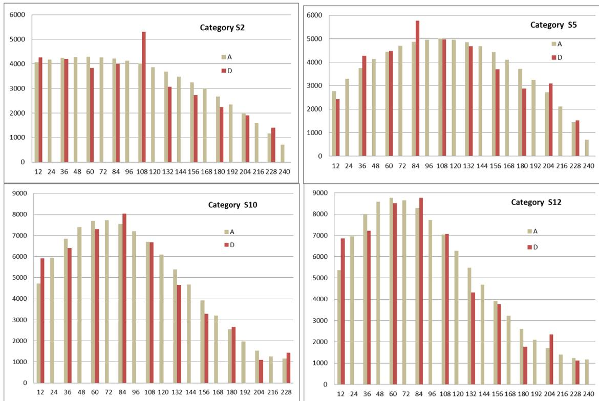
Fig. 3. *PM1 and PM2 values vs. vehicle operation time (in months), in a few categories of engine cubic capacity; the PM1 and PM2 values, denoted by letters A and B, respectively, have been specified in kilometres per month [km/m]*
