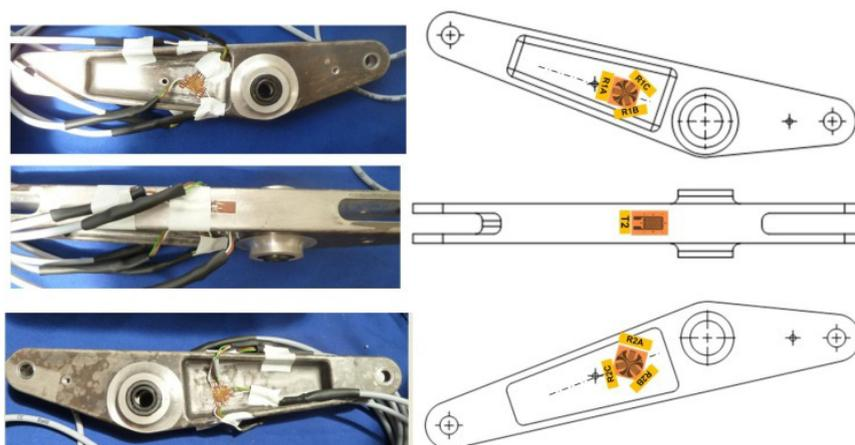
Fig. 7. Strain gauge points installation
