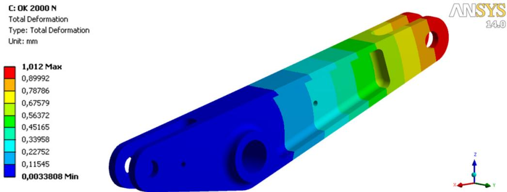
Fig. 6. Total displacement of the control – system lever, isometric view
