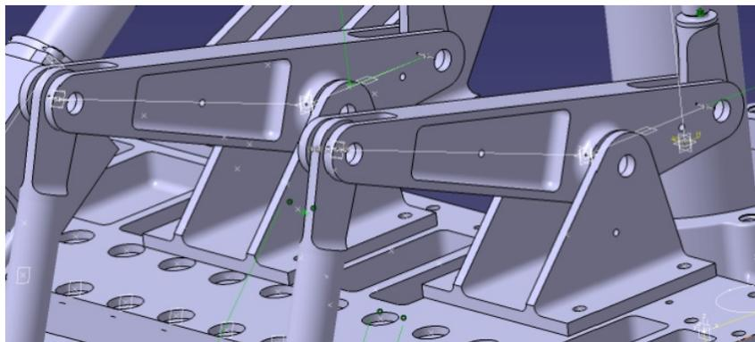
Fig. 1. Control – system levers 3D model in Catia
