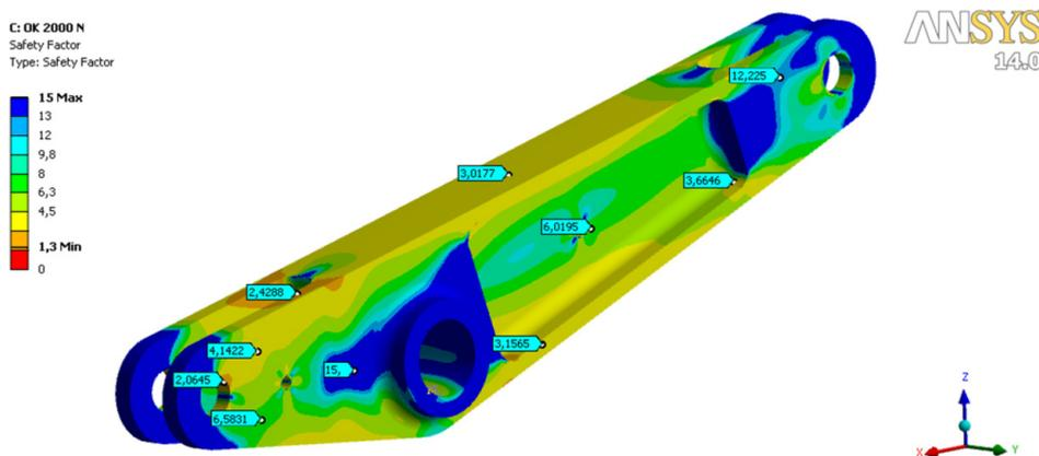
Fig. 5. Distribution of the safety factor on the control – system lever
