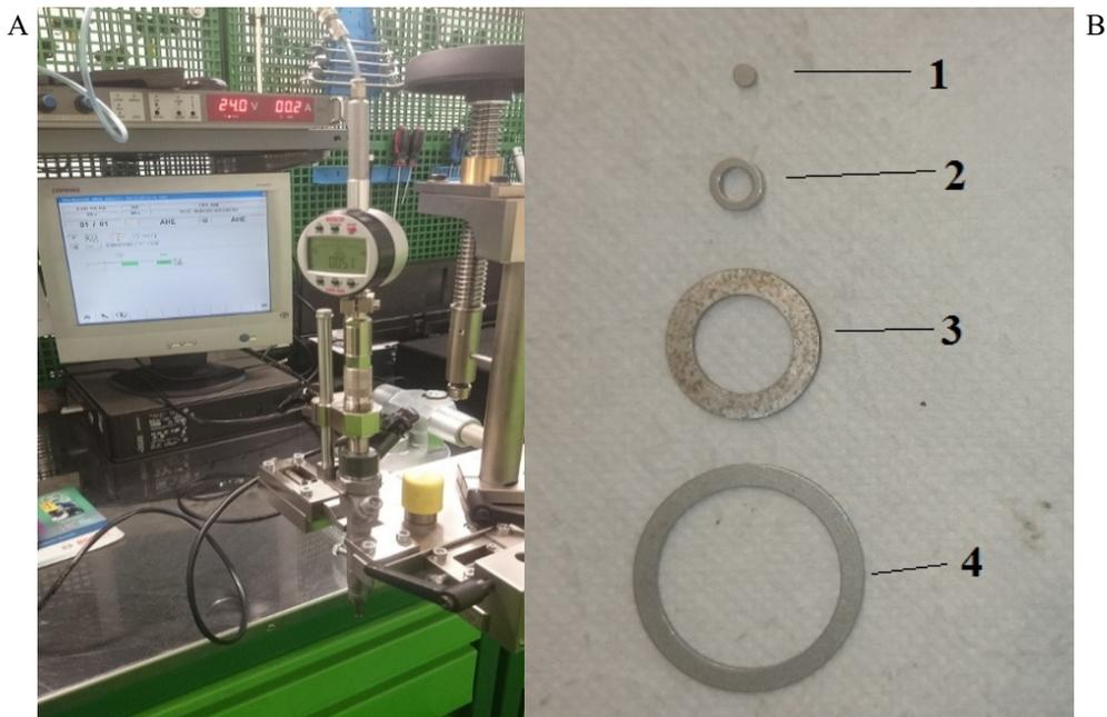
Fig. 9. Steering valve adjust process (A). Adjust pads (B): 1 – VL dosage, 2 – LL dosage, 3 – AHE (range of work injector valve), 4 – initial dosage
