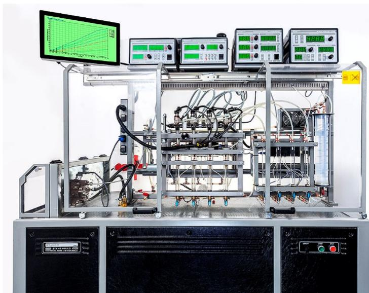
Fig. 6. Test bench for testing fuel injectors STPiW – 3
