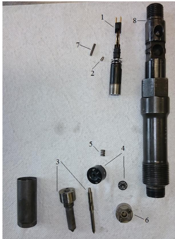
Fig. 4. Delphi fuel injector subdivided into its components: 1 – solenoid, 2 – regulation all dosages clot in solenoid, 3 – nozzle, 4 – steering valve, 5 – spring over needle, 6 – washer over nozzle unit, 7 – spring in solenoid, 8 – injector body
