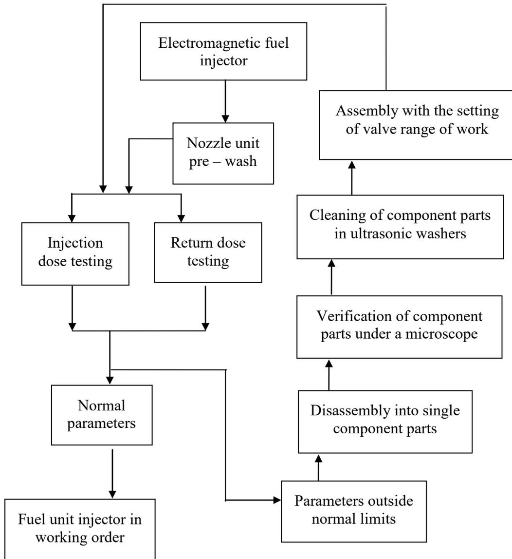
Fig. 5. Fuel unit injector testing and repair procedure
