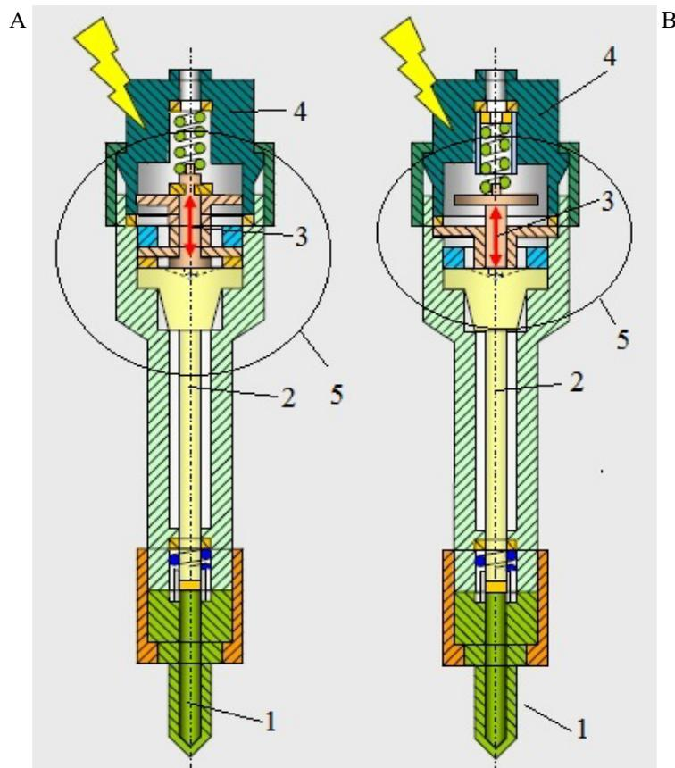
Fig. 3. Bosch gen. 1.0, 2.0, 2.2 (A), gen. 2.1 (B) fuel injector subdivided into its areas: 1 – nozzle unit, 2 – fuel injector valve, 3, 4 – electromagnetic solenoid, 5 – injector steering area [11]
