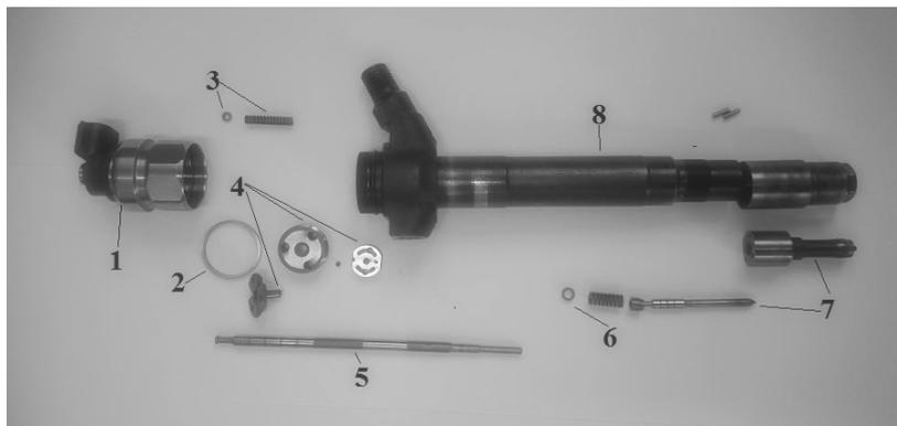
Fig. 1. Denso fuel injector subdivided into its components: 1 – solenoid section, 2 – RLS slit regulation washer, 3 – solenoid section elements, 4 – steering valve section, 5 – piston section, 6 – regulation washer, 7 – nozzle unit, 8 – injector body
