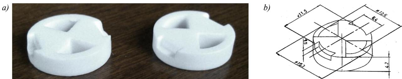
*Fig. 4. Valve sealing lapped during the tests*
