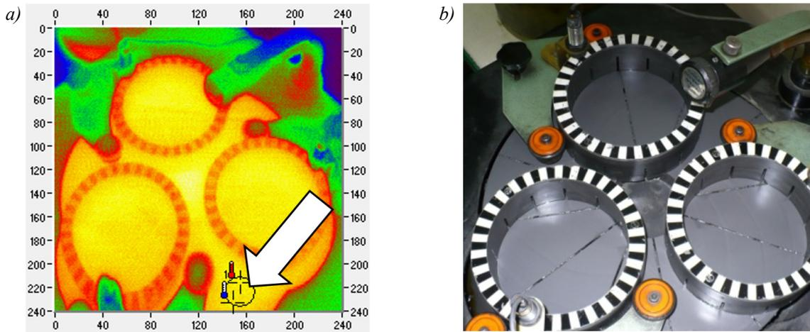
Fig. 6. ABRALAP 380 executory system: a) the thermographic camera view, b) photo camera view
