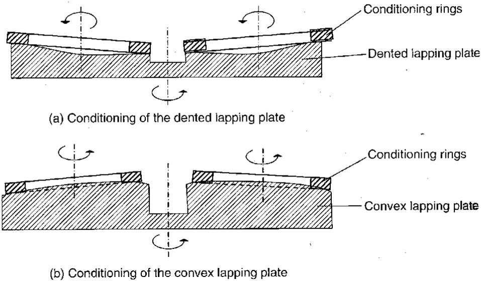
*Fig. 3. Conditioning methods of the lapping plate with a conditioning rings [10]*
