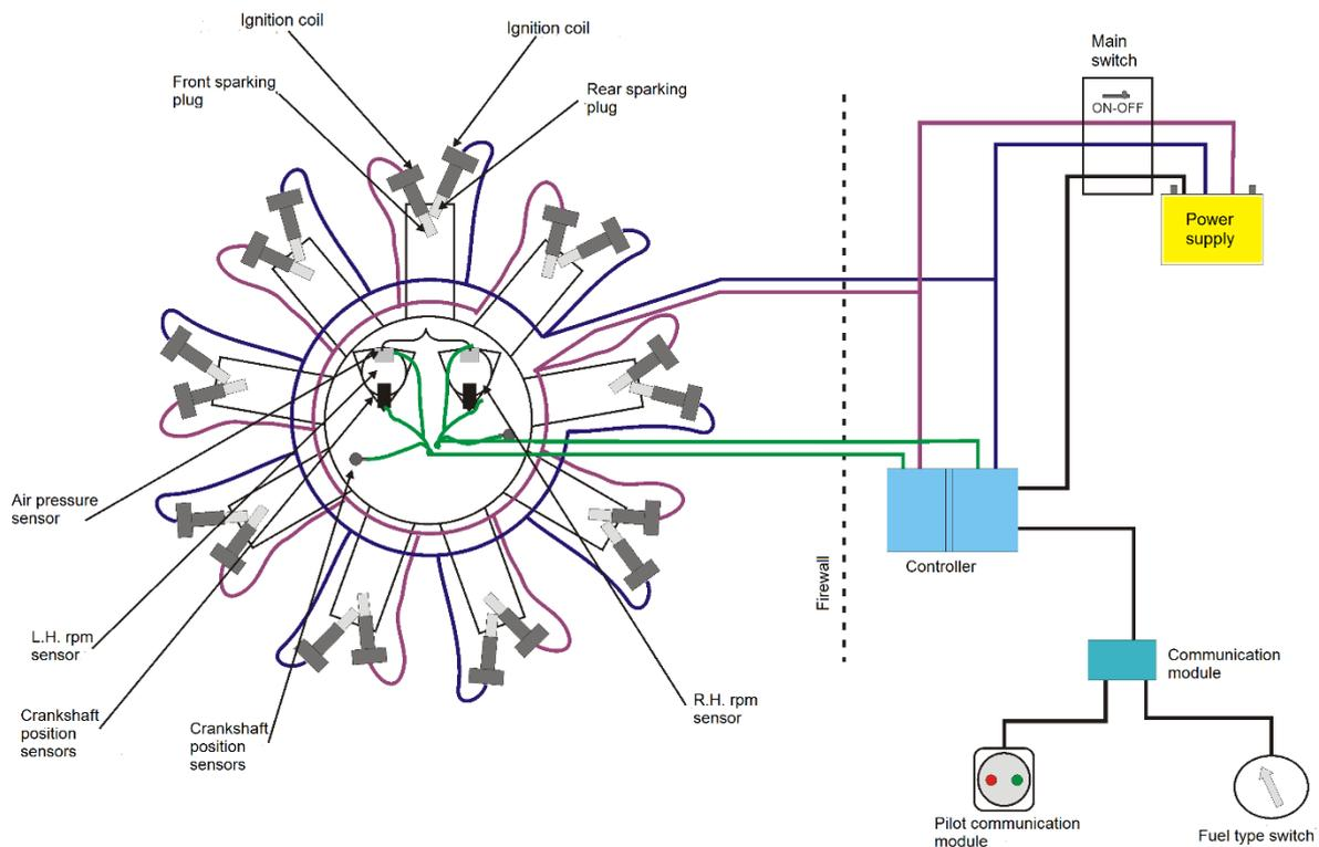
*Fig. 2. Electronic ignition system*
