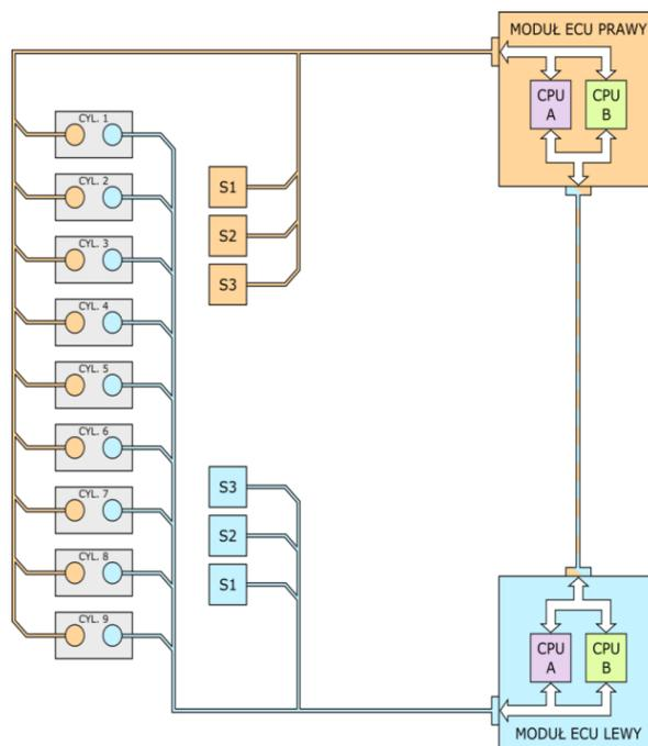
Fig. 3. Setup of control units of the ignition system
