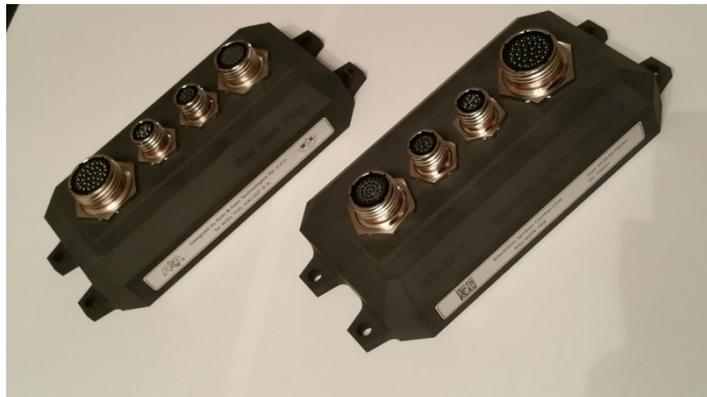
*Fig. 4. Original design of ignition system control units*
