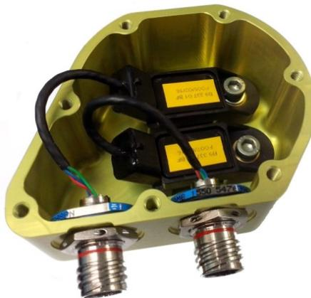
*Fig. 5. Air pressure sensors in custom-made protective casing*
