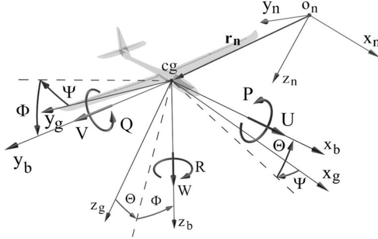
Fig. 2. Navigation, gravity and airplane coordinate system
