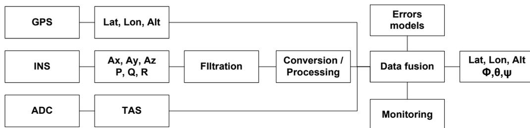
Fig. 1. System architecture
