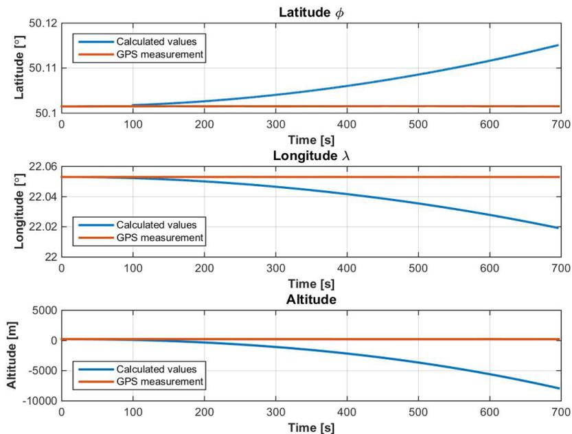
Fig. 5. Calculated position based on filtered accelerations
