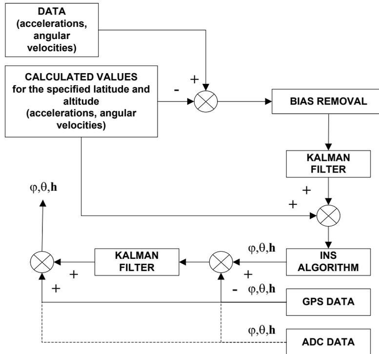
Fig. 3. Filtration algorithm
