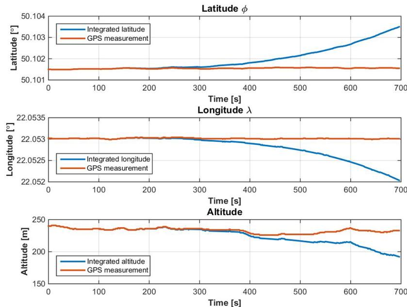
Fig. 6. Fused INS / GPS position
