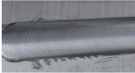
Fig. 9. An example of friction stir welded joint with correct temperature – lack of welding defects
