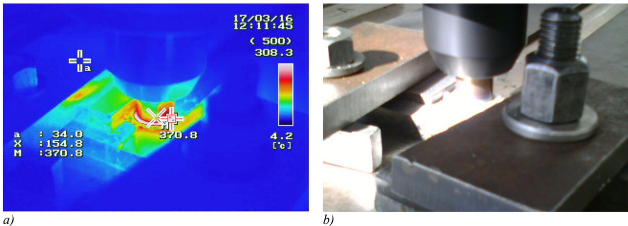
Fig. 5. Thermogram (a) and visual picture (b) of FSW process during plasticizing – sufficient temperature to start welding (370.8°C)
