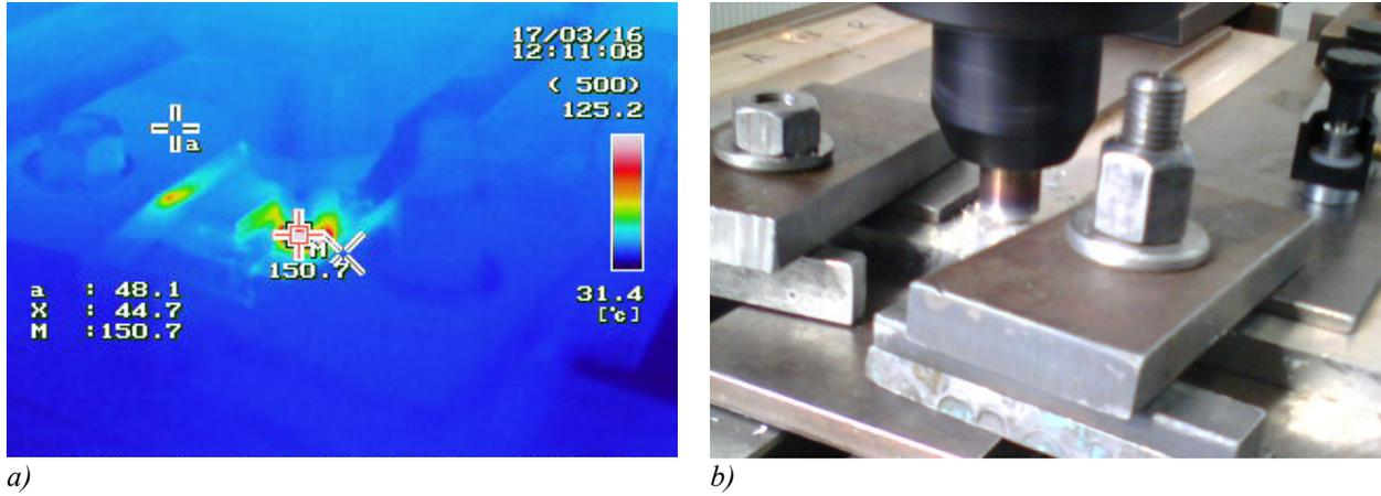
Fig. 3. Thermogram (a) and visual picture (b) of FSW process during plasticizing – relatively low temperature in contact point (150.7°C)
