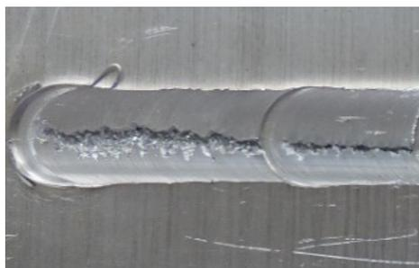
Fig. 8. An example of friction stir welded joint with too high temperature – visible welding defects
