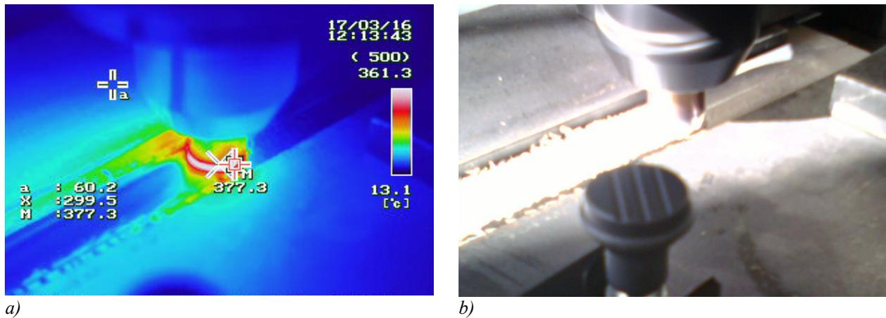
Fig. 6. Thermogram (a) and visual picture (b) of FSW process during welding – correct temperature allowing obtain high quality of joint (377.3 °C)
