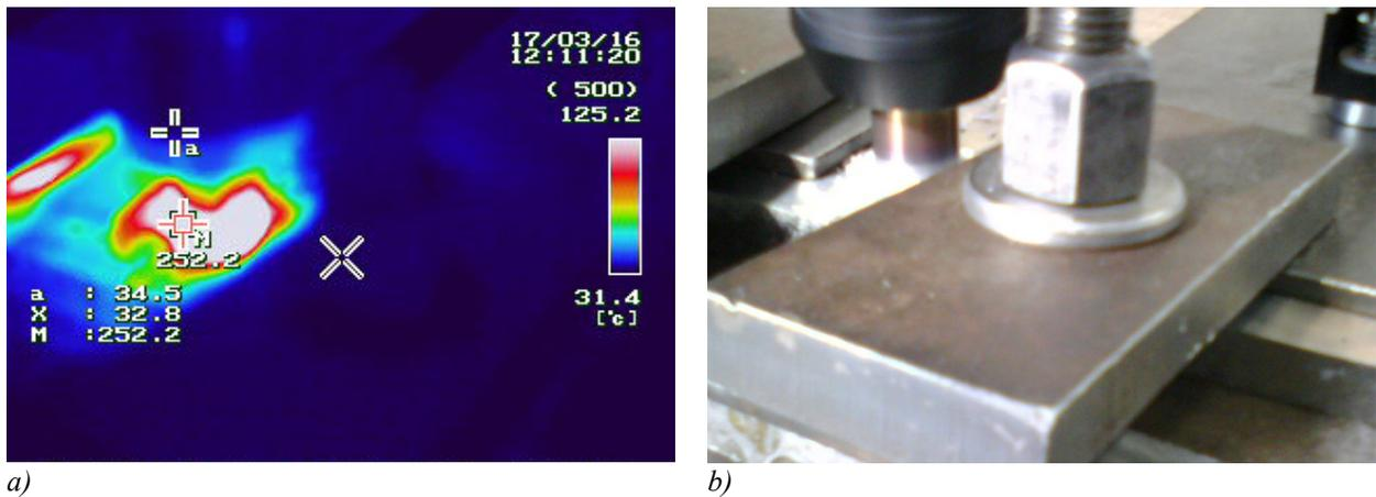
Fig. 4. Thermogram (a) and visual picture (b) of FSW process during plasticizing – medium temperature in contact point (252.2°C)
