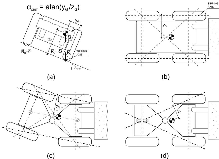
Fig. 1. Tipping axes: a – the method of determining the critical ground inclination angle, b – tipping axes in the vehicle with a rigid frame, c – dislocation of the gravity centre at the twisted articulation, d – tipping axes in the vehicle with the self-aligning bridge
