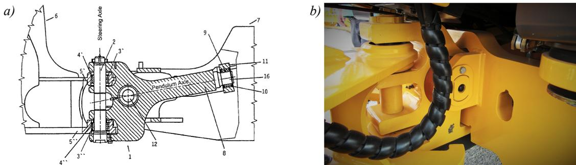
Fig. 4. An exemplary solution of articulation joint and the inclined axis' oscillation joint between bodies of a vehicle applied by Volvo; a – illustration from the patent [13], b – an example of application (own data)
