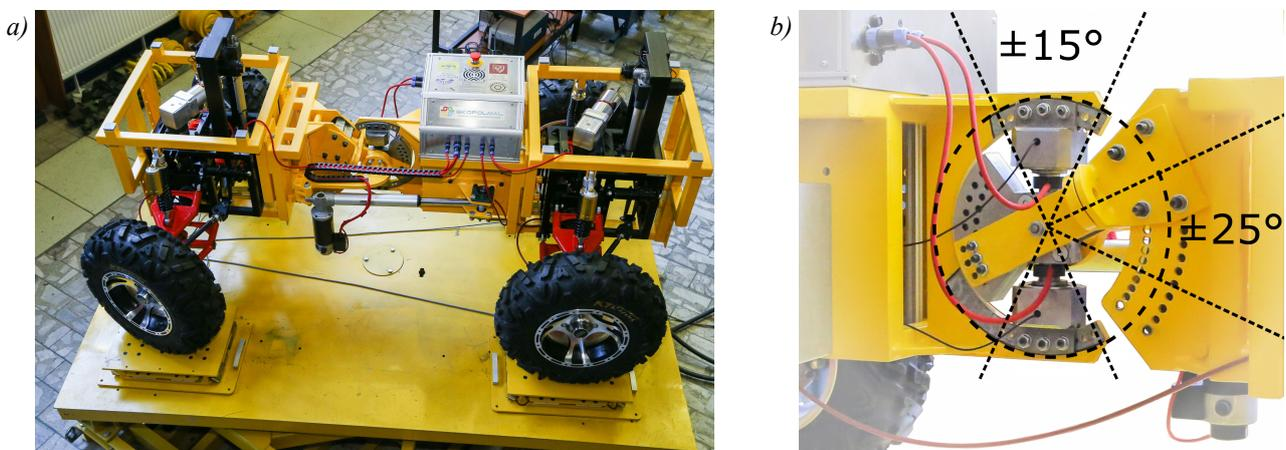
Fig. 6. The innovative universal test vehicle of adaptable structure and properties of the undercarriage system at the tilting-rotary platform equipped with 3-axial measurement plates
