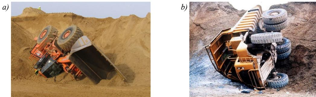
Fig. 3. Examples of losing the roll-over stability in the machine for ground works during their operation: a – articulated bucket loader [14], b – dump with the so called rigid frame [15]
