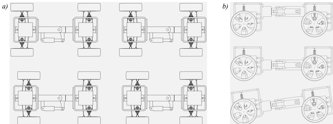
*Fig. 7. Special construction of the developed universal test vehicle enables changes in many geometrical parameters of the undercarriage system such as: a – wheelbase and the position of the articulation joint, b – height and location of the crossing point of the articulation joint axis with oscillation joint axis.*
