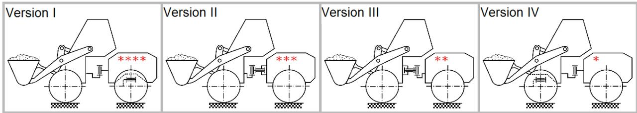
Fig. 2. The impact of the oscillation joint localisation with horizontal axis on roll-over stability of the articulated wheel bucket loader (greater number of stars indicates for higher roll-over stability) [4]
