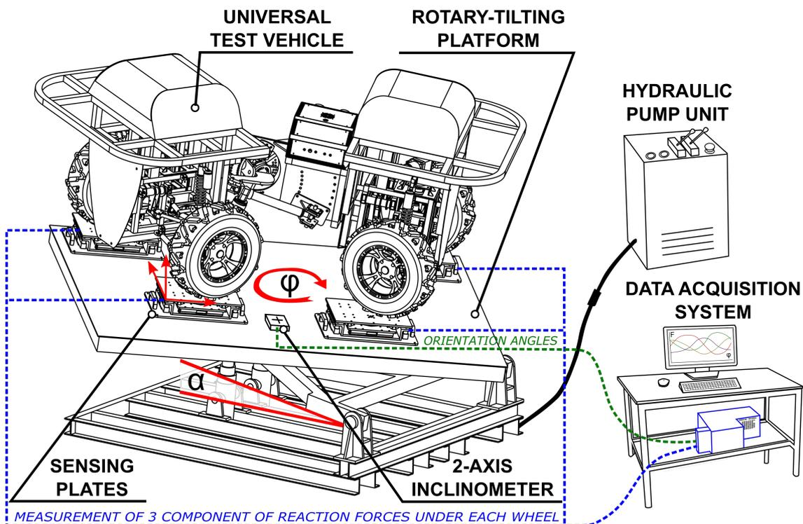
Fig. 5. Schematic of the stand developed for tests of the roll-over stability of wheeled vehicles of arbitrary structure and properties of the undercarriage system
