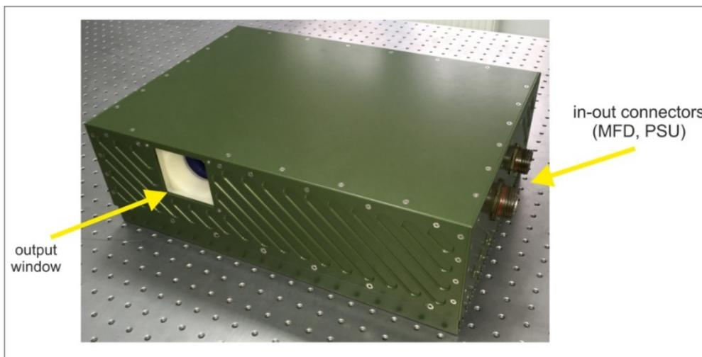
*Fig. 8. 3D scanning system. View of prototype in the housing*
