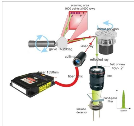
*Fig. 3. Schematic structure of 3D scanner*
