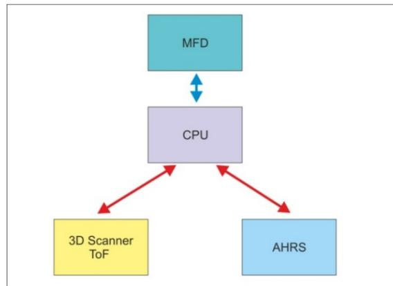
Fig. 5. Schematic structure of the 3D landing system
