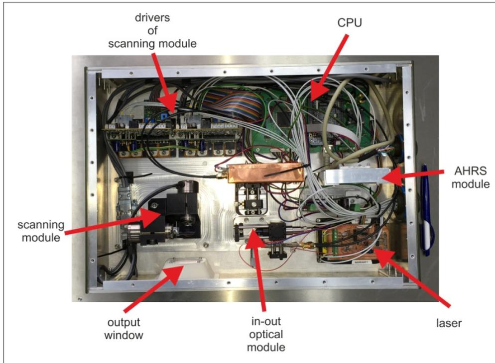
*Fig. 7. Prototype of 3D scanning system inside*
