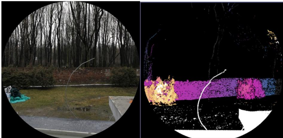
Fig. 10. Outdoor scanning, range – 30 m. Left – photo, right – 3D scan
