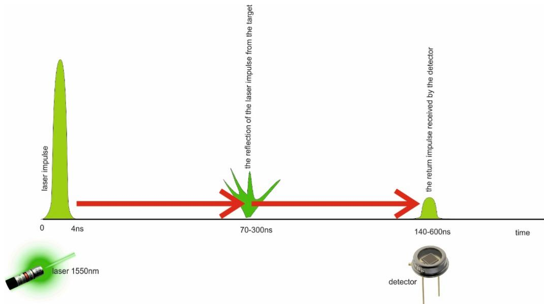
Fig. 2. Timing of the process “generate impulse-reflection-receiving”
