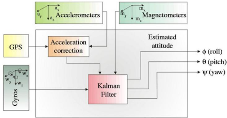
Fig. 4. Schematic structure of the AHRS system
