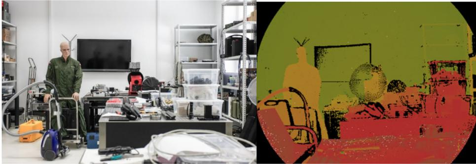
Fig. 9. Indoor scan, range 5 m. Left – photo, right – 3D scan
