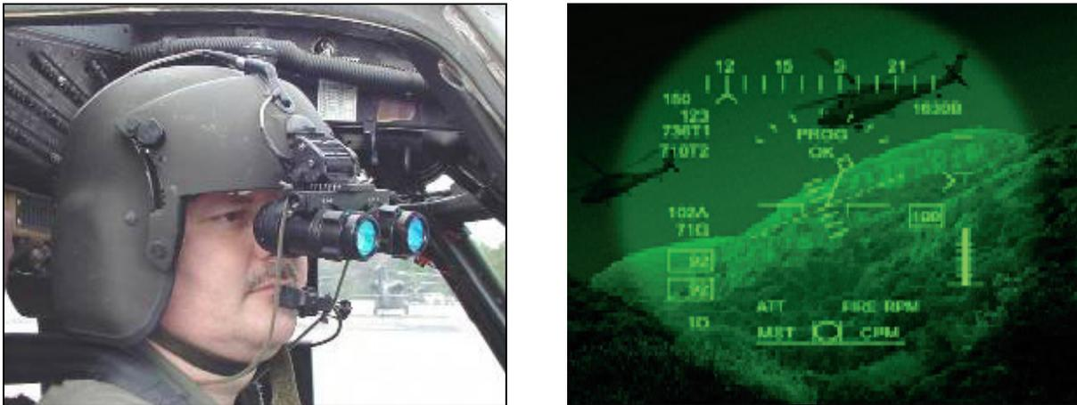
Fig. 1. The ANVIS Helmet-Mounted Display System for AH-1 military helicopters [8]
