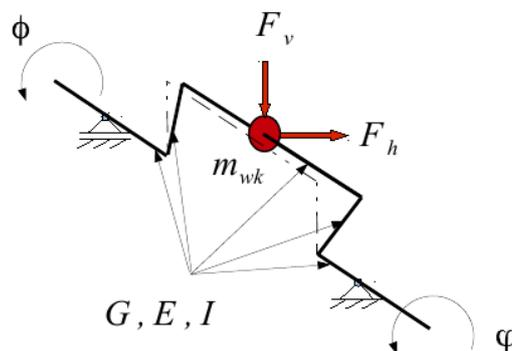
Fig. 1. The model of the crankshaft of the one piston
