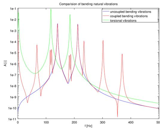
*Fig. 8. Comparison of natural displacements of torsional and bending vibrations of the model of the crankshaft with and without coupling*
