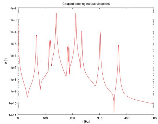
*Fig. 7. Bending vibrations of the crankshaft of the system with a coupling*
