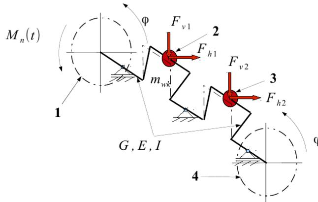
Fig. 2. The model of the crankshaft with two pistons
