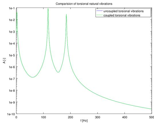
*Fig. 6. The spectrum of natural displacements of torsional vibrations of the model of the crankshaft with the coupling*
