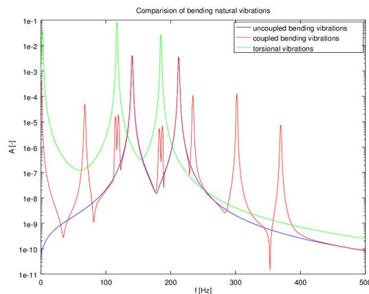
*Fig. 8. Comparison of natural displacements of torsional and bending vibrations of the model of the crankshaft with and without coupling*
