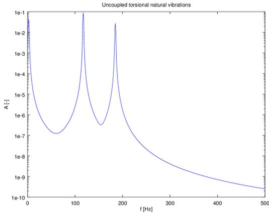
*Fig. 4. The spectrum of natural displacements of torsional vibrations of the model of the crankshaft without the coupling*
