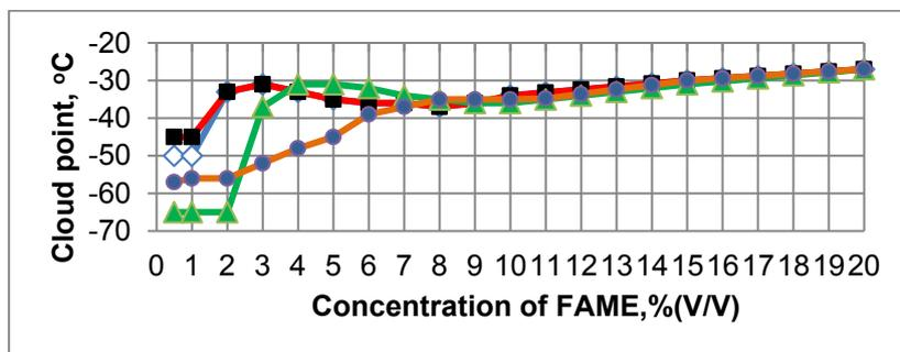
Fig. 5. Cloud point and freezing point change with the increase of FAME concentration in jet fuel; each line represents blend of jet fuel (two kinds of this fuel) and FAME (from two plants) [5]
