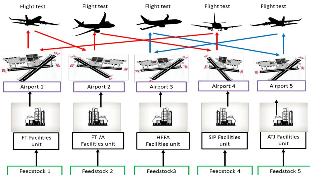
Fig. 5. Technical-logistic problem 1: the same aircraft will be supply with various biojet fuels at various airports
