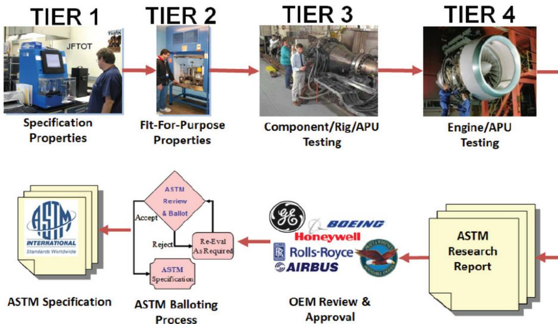
Fig. 3. The algorithm of new synthetic biojet fuels authorization according to ASTM D 4054 standard [8]
