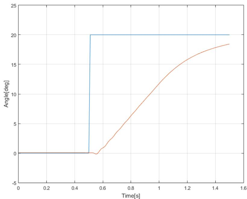
*Fig. 5. Step response with small P and I value*
