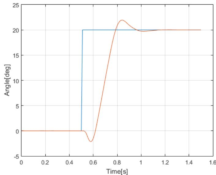
*Fig. 4. Step response with large P value*
