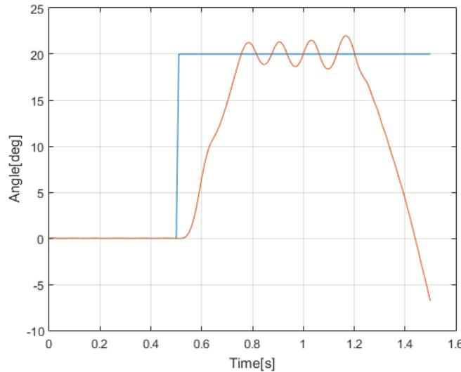
Fig. 6. Step response with large P and D
