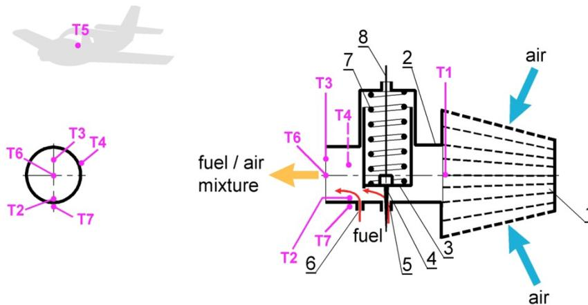
Fig. 1. The diagram showing locations of thermocouples used during the in-flight tests: 1 – air filter, 2 – carburettor body, 3 – slide throttle, 4 – needle, 5 – main jet, 6 – idle jet, 7 – slide throttle spring, 8 – slide throttle-controlling bowden, T1...T7 - thermocouples
