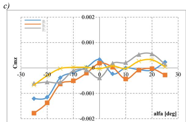
Fig. 7. The influence of: the passive protection or lack of protection, and stabilizer or lack of stabilizer on: a)  $C_x$  drag force coefficient, b)  $C_y$  side force coefficient, c)  $C_z$  lift force coefficient, of the helicopter fuselage model for various angles of attack and the sideslip angles  $\beta = 0$  deg
