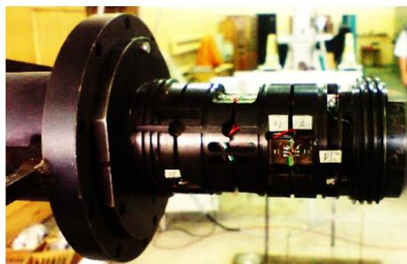
Fig. 4. HWG-6 six-components internal strain gauge balance used for the helicopter fuselage model tests
