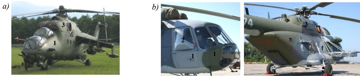
Fig. 1. The Polish Mi-24W (a) and the Czech Mi-171Š (b) gunship helicopter with the additional protection of cockpit (1), windows (2) and the engine (3) against the perforation with API projectiles 7.62 mm (a) and 7.62-12.7 mm (b)
