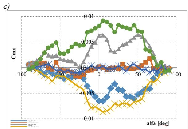
Fig. 5. The influence of the passive protection and lack of protection on: a)  $C_x$  drag force coefficient, b)  $C_y$  side force coefficient, c)  $C_z$  lift force coefficient, of the helicopter fuselage model for various angles of attack and the sideslip angles  $\beta = -10, 0, 10$  deg
