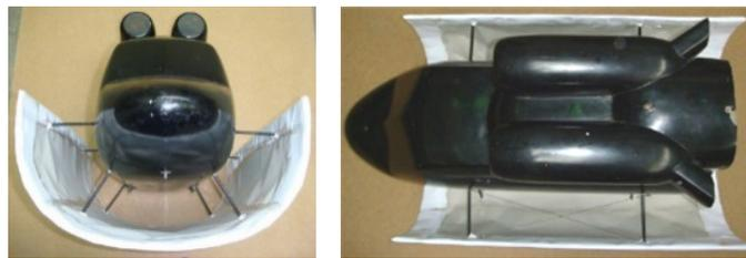
Fig. 2. The fuselage of the *Sokol* helicopter model with protection
