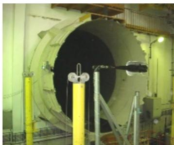
Fig. 3. The Sokol helicopter model with the passive armour model in the wind tunnel
