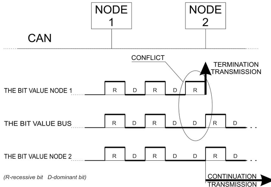
Fig. 1. example of CAN arbitration
