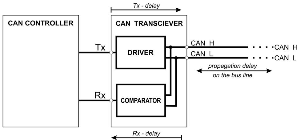
Fig. 2. Scheme of CAN transceiver
