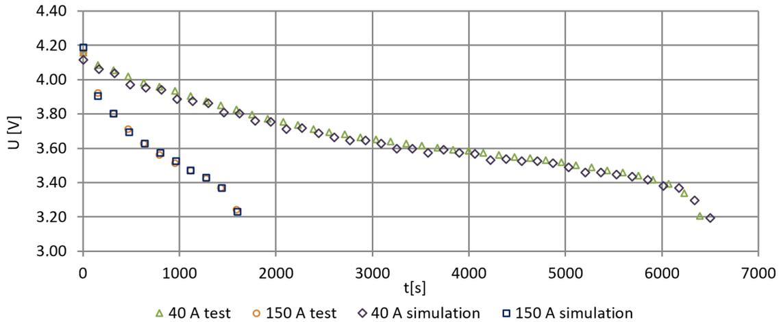
Fig. 6. Comparison battery characteristics with simulation model
