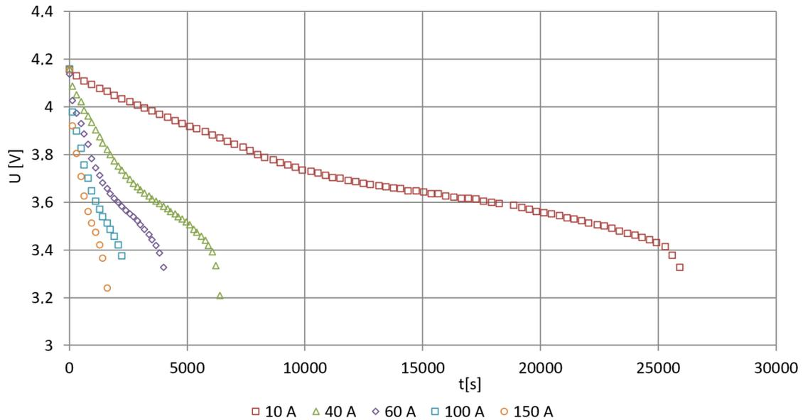
Fig. 2. Diagram of time discharging of the cell, depend on current current
