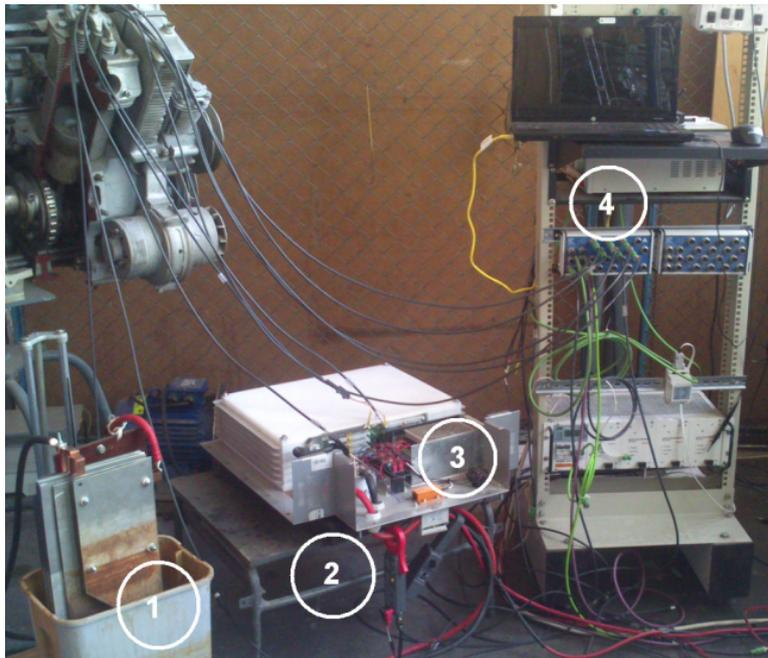
Fig. 1. Test stand for battery discharging: 1 – water resistor, 2 – current clamps, 3 – battery with voltage probes connected, 4 – acquisition computer with data logging card
